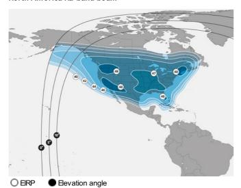
The inclined all Ku-band satellite has a comprehensive coverage of the United States, Gulf of Mexico and the Caribbean. It enables a range of services which includes video contribution and distribution, VSAT networks and broadband access.
