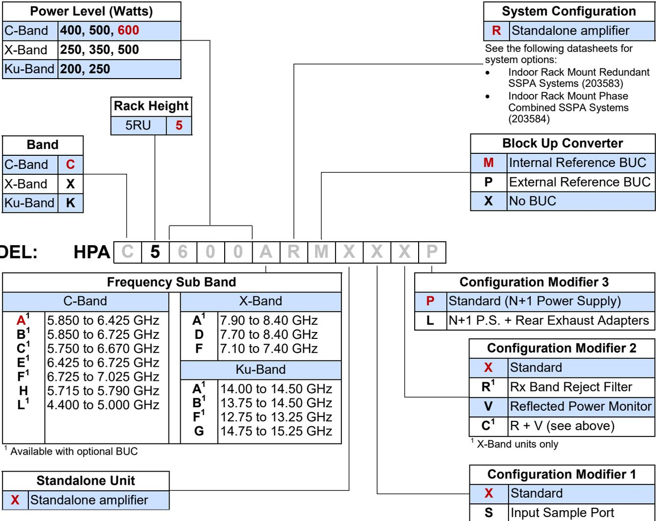
**Example** - A standalone 600W GaAs C-Band 5RU Rack Mount SSPA with standard N+1 external power supply and an optional internal reference block up converter is part number: **HPAC5600ARMXXXP**.
