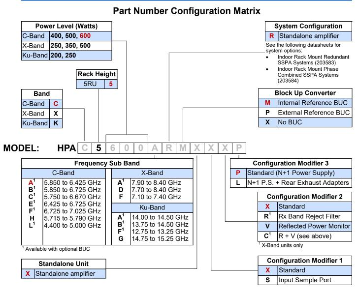
**Example** - A standalone 600W GaAs C-Band 5RU Rack Mount SSPA with standard N+1 external power supply and an optional internal reference block up converter is part number: **HPAC5600ARMXXXP**.
