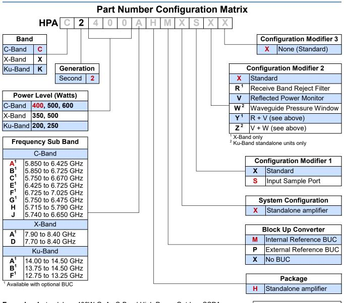
**Example** - A standalone 400W GaAs C-Band High Power Outdoor SSPA an optional input sample port and optional internal reference block up converter is part number: **HPAC2400AHMXSXX**.
