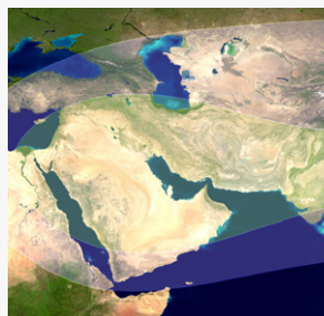
T3 Beam EIRP Contours
