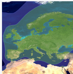
T3 Beam EIRP Contours
