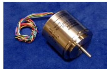
The 7200 system offers 3 options for position encoding accuracy. Standard single speed brushless size-11 resolvers (above); 2-speed brushless size-20 resolvers (above right); and optical encoders (right).
