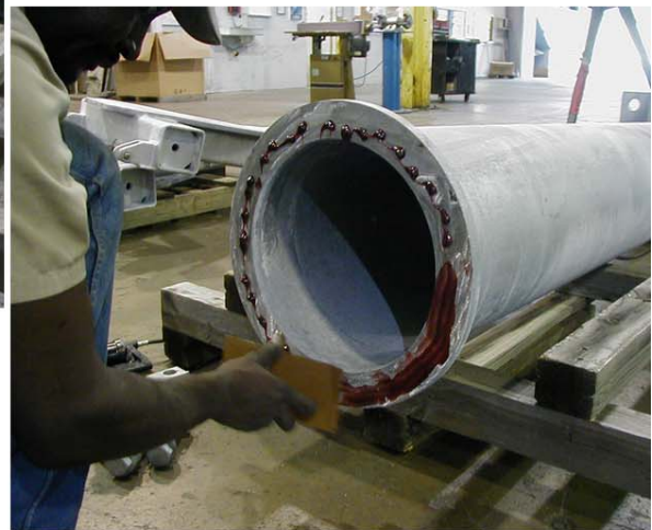
Figure 2-3. Application of Grease to Top Surface of Pedestal Post
