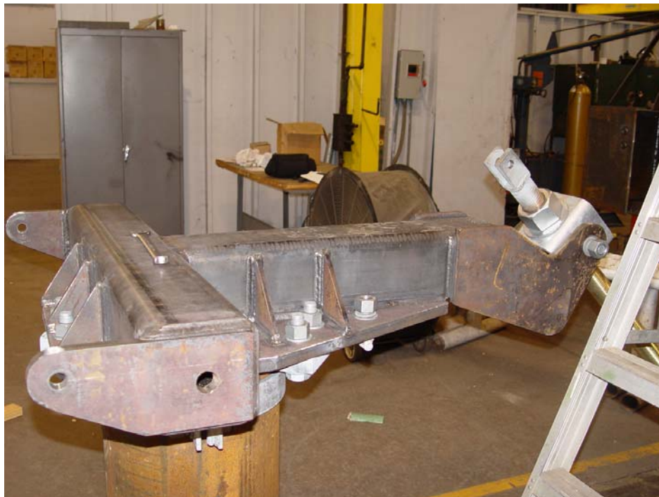
Figure 2-7. Turning Head Installed
