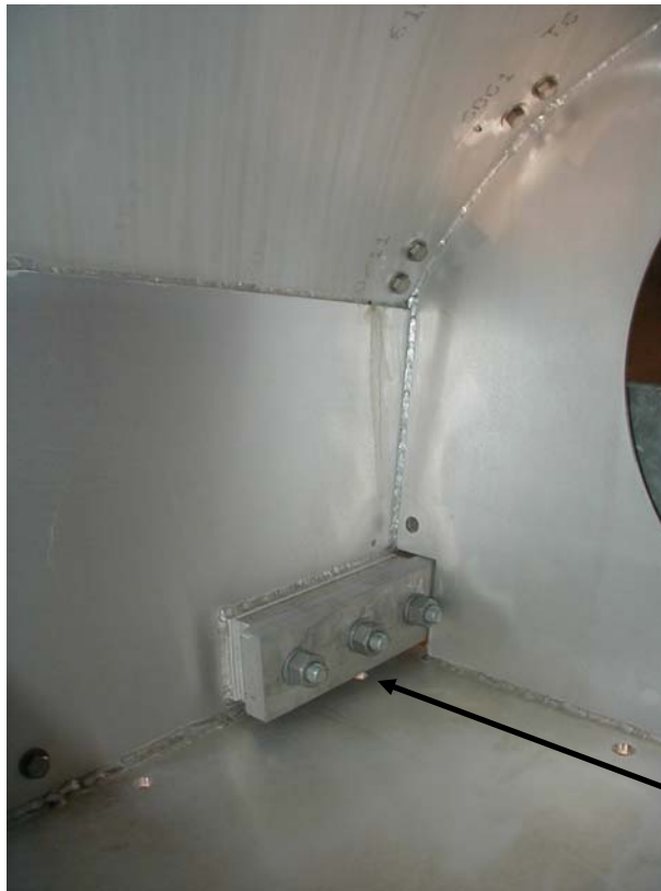
Figure 2-12. Elevation Axis Lug and Spacer – Inside Hub
