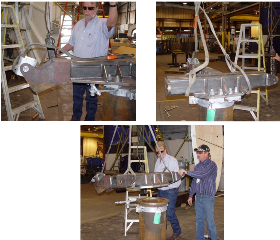
Figure 2-4. Lifting and Installation of the Pedestal Turning Head
