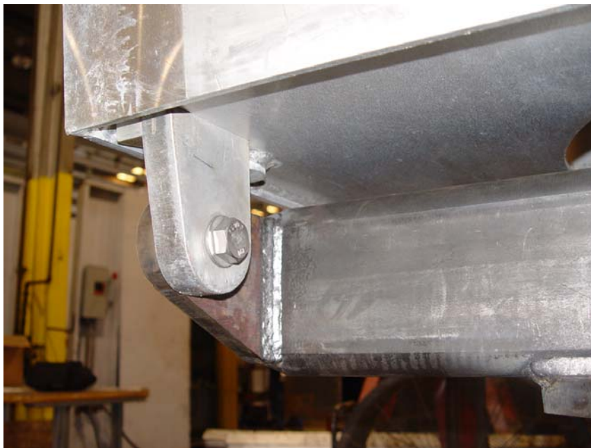
Figure 2-15. Hub Installed on Turning Head
