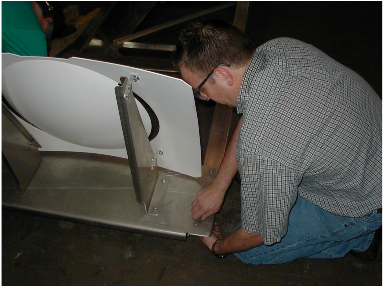
Figure 2-35. Attaching the Subreflector
