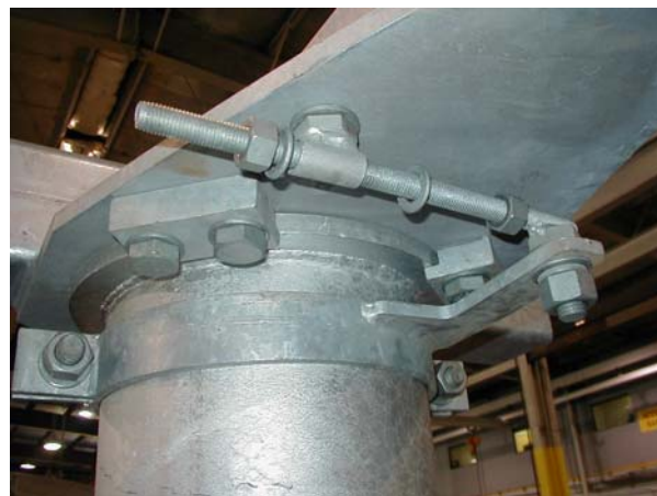
Figure 2-10. Azimuth Adjustment Rod
