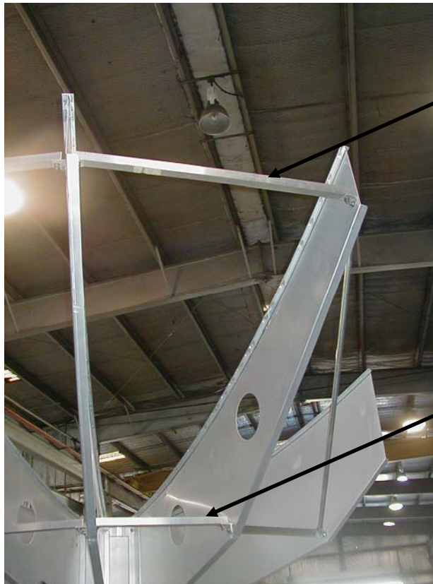
Figure 2-26. Lacing Between Radial #2 and #3 and Between #1 and #2
