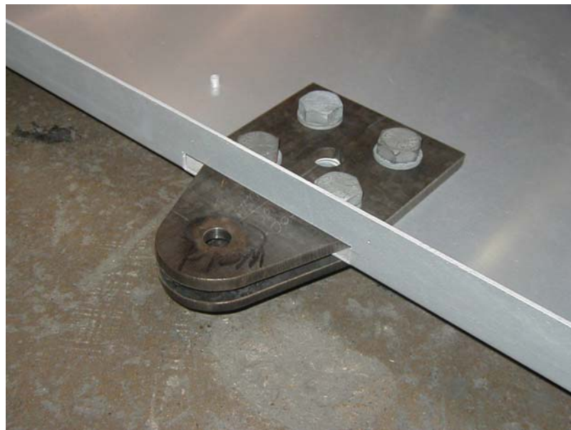
Figure 2-16. Radial Beam Lugs
