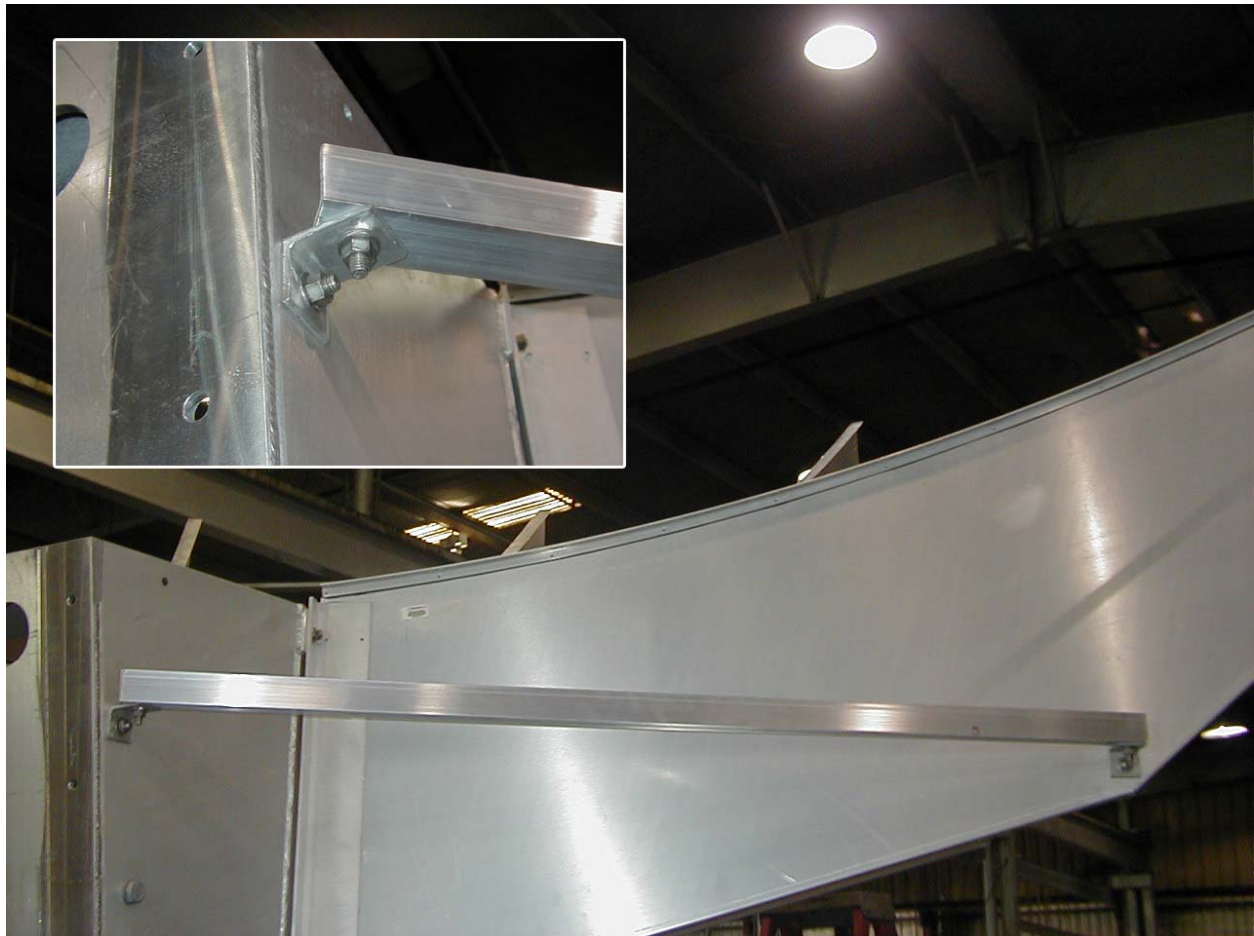
Figure 2-24. Lacing Between Hub and Radial #4
