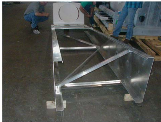
Figure 2-33. Feed Boom Braces
