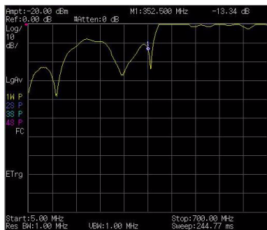
Figure 23 Measuring the Return Loss of the Filter
