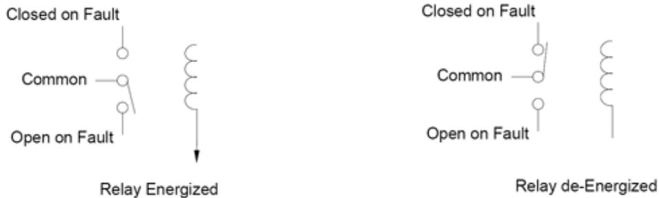
Figure 2: Parallel I/O Form-C Relay
