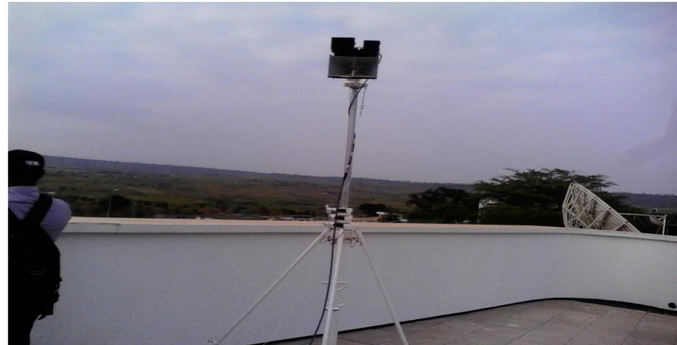
Installation and operation a GNSS ground station allows to increase the local accuracy precise point positioning of consumer navigation from units of meters (2-5 m) to tens of centimeters (10-30 cm), and open again an opportunity for capacity building.
