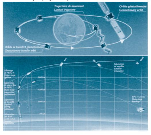
Standard Ariane 5 trajectory for geostationary transfer orbit
