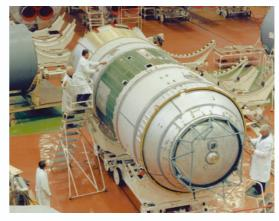
nozzles provide three-axis flight control. The third stage engine nominally burns for 240 seconds. After engine cut-off and separation of the fourth stage, the third stage performs an avoidance maneuver by opening an outgassing valve in the liquid oxygen tank.
