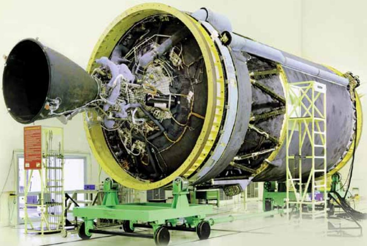
C25 Cryogenic Stage with 20 tonne thrust Cryogenic engine at stage Preparation Facility
