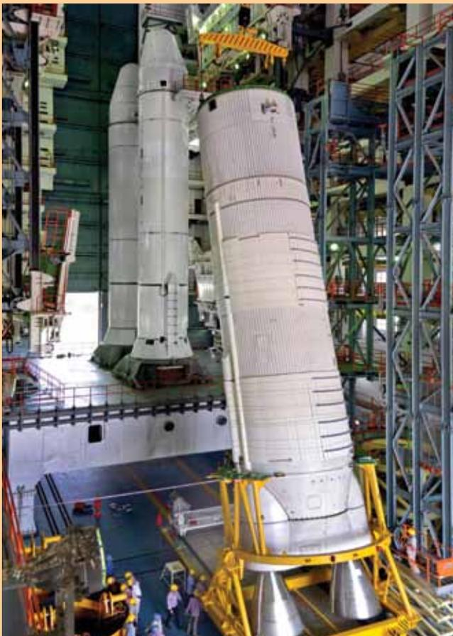
Hoisting of L110 during vehicle integration
