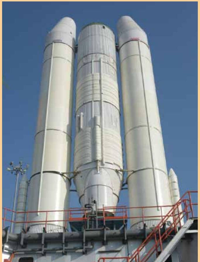
S200 strap-ons integrated with Core L110 liquid Stage
