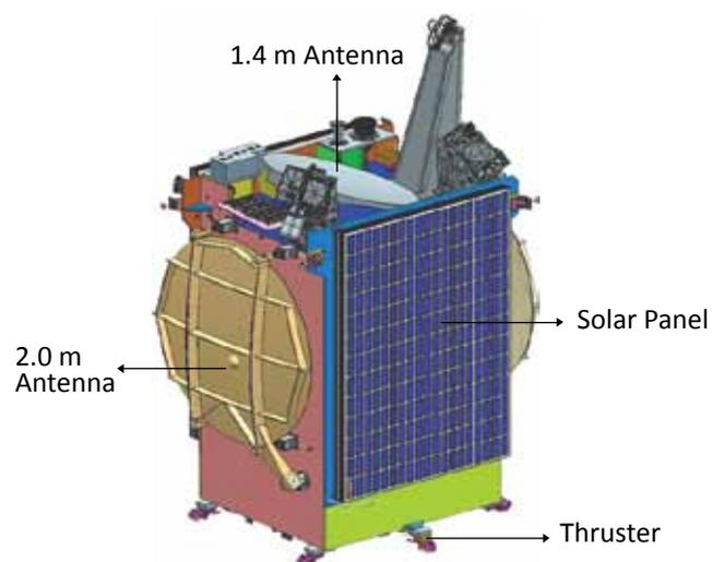
GSAT-19 with solar panel and antennas in folded position
