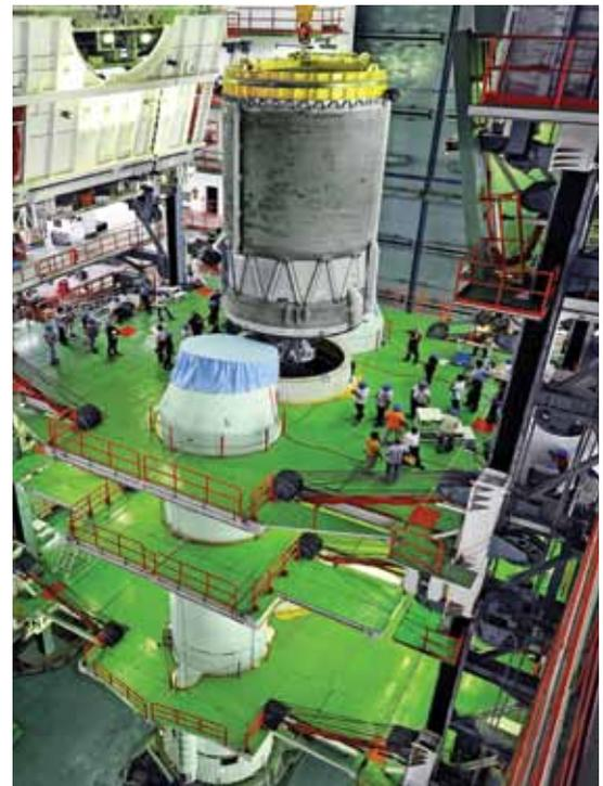
Integration of C25 stage in progress at Vehicle Assembly Building
