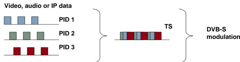
Figure 58- DVB-S used to Carry Video, Audio and Data in an MPEG Transport Stream
