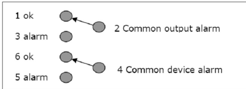
Figure 21 - Contact Closure Alarm Connections of the EL970
