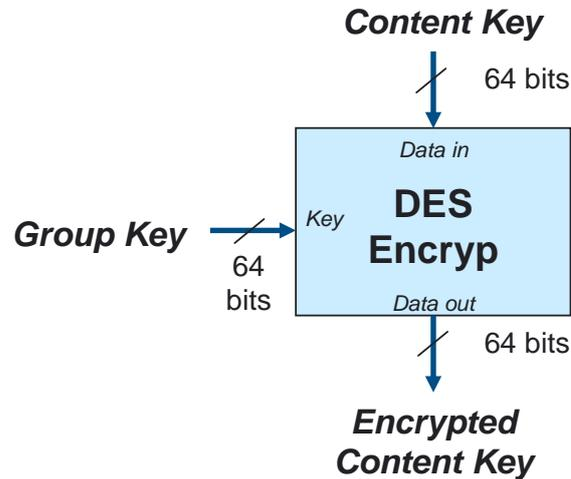
Figure 121 - Process to Encrypt a Content Key with a Specific Group Key in 64-bit Mode
