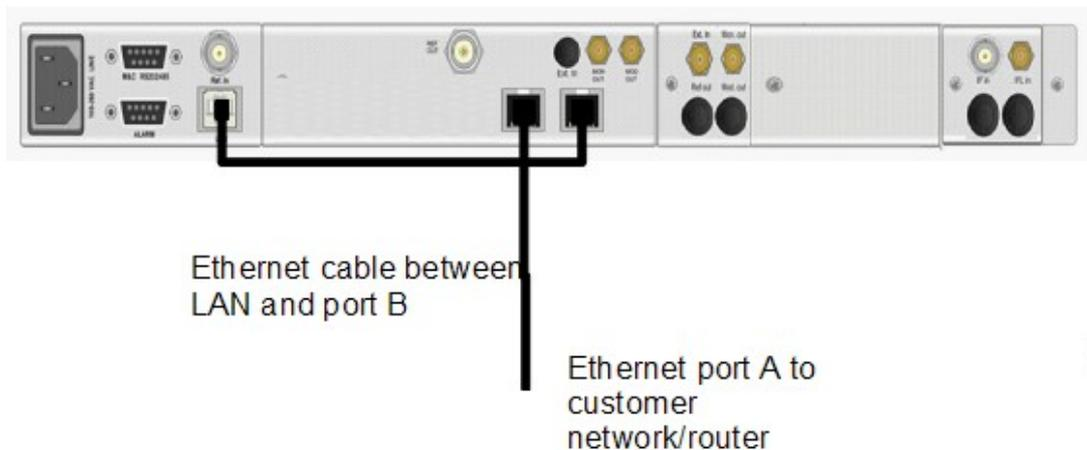
**Figure 100 – Loopback Management Physical Connection**
