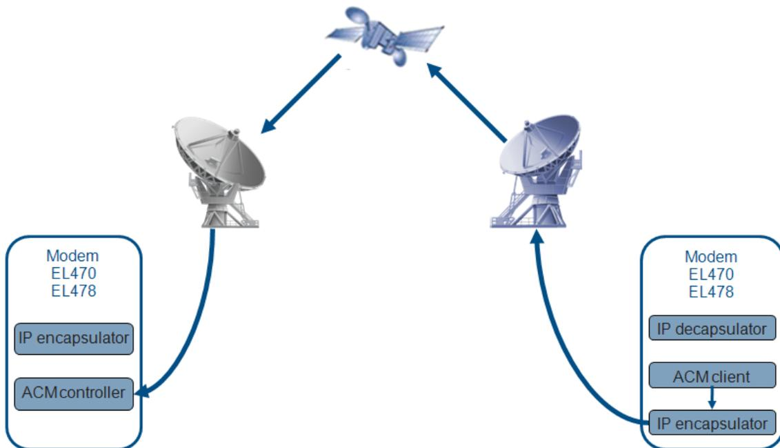
Figure 86 - In-band Return Signalling
