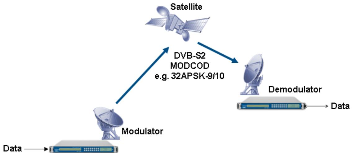
Figure 70 – Data Transmission via Satellite
