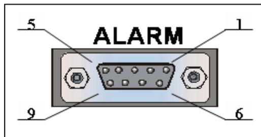
Figure 19 - Contact Closure Alarm Outputs
