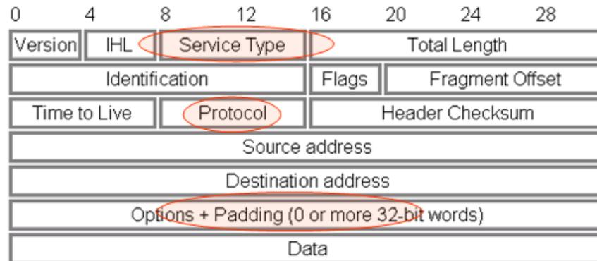
**Figure 99 – IP Datagram Format (IPv4)**
