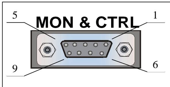
Figure 18 - Serial Monitoring and Control Connector
