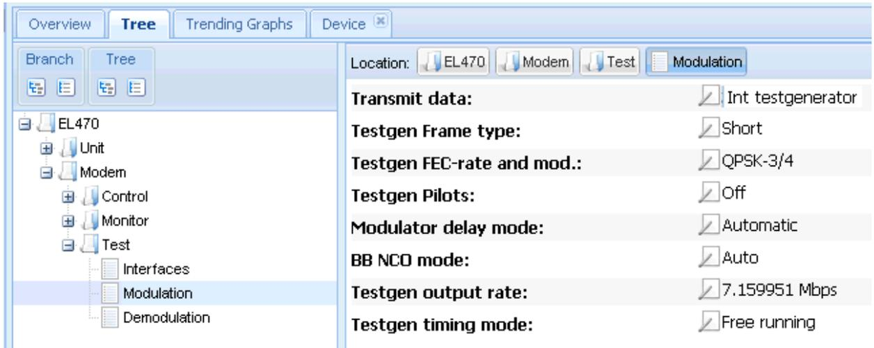
Figure 108- Modulator Test Generator
