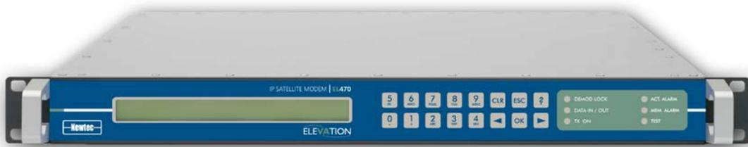
Figure 11 – EL470 IP Satellite Modem Front Panel
