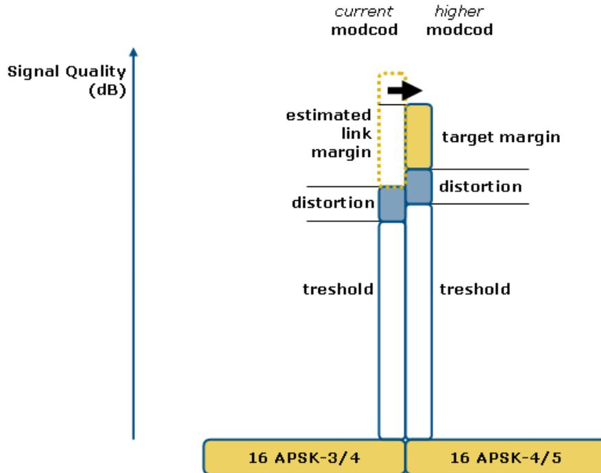
Figure 78 - Selecting a higher ModCod Based on Estimated Link Margin
