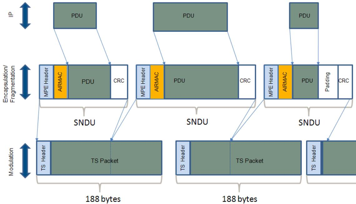
Figure 65 - MPE Encapsulation of IP Packets
