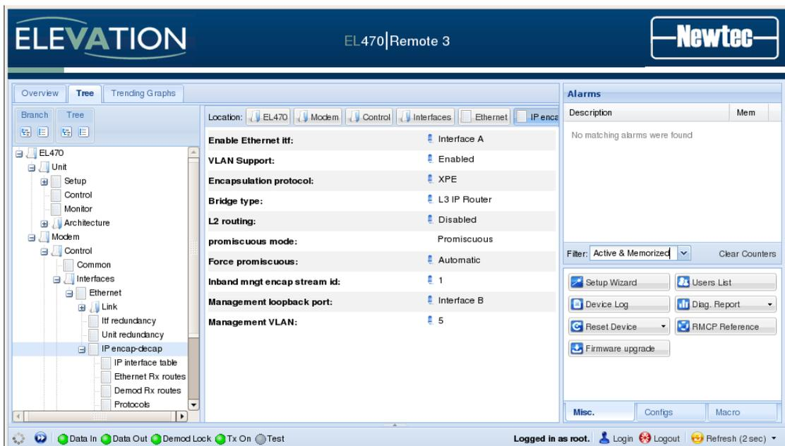
Figure 101 –Management Loopback Port and Management VLAN
