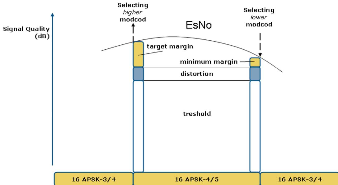
Figure 77 - Selecting the Optimal ModCod Based on EsNo
