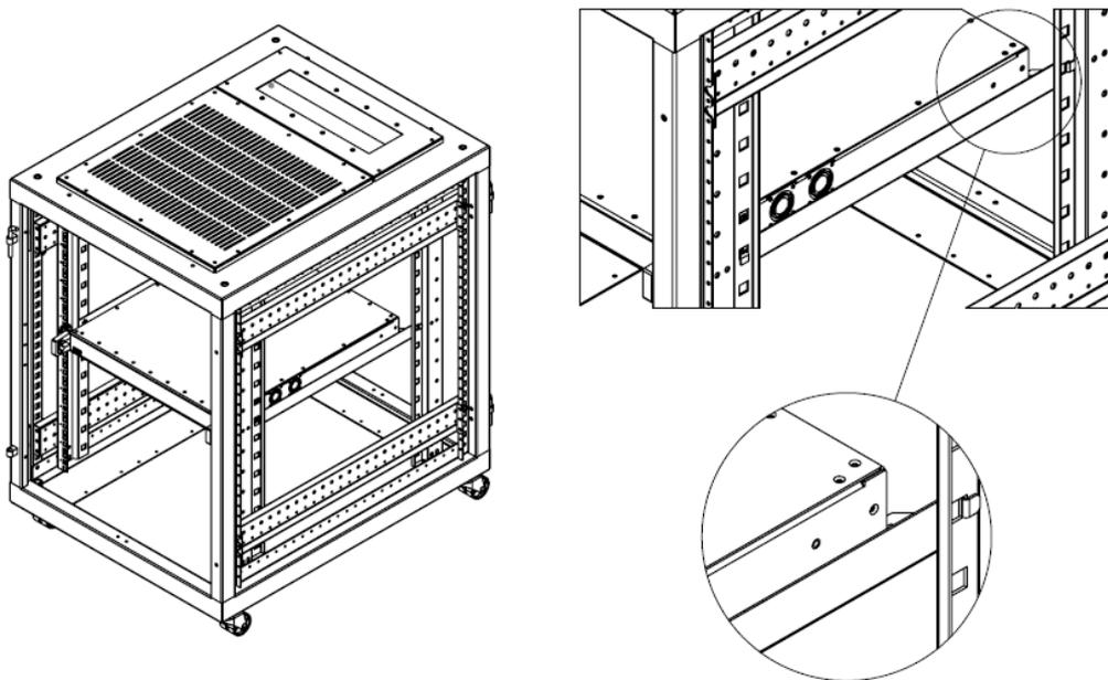
Figure 8 - Mounting with L-Profiles
