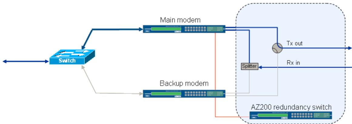
Figure 102 - Example of Equipment Redundancy Configuration
