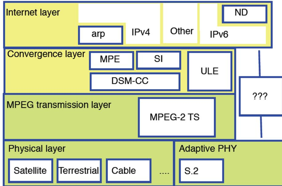
Figure 67- Modulation and Encapsulation Layered Model
