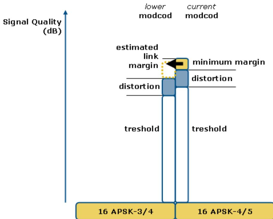
Figure 79 - Selecting a Lower ModCod Based on Estimated Link Margin
