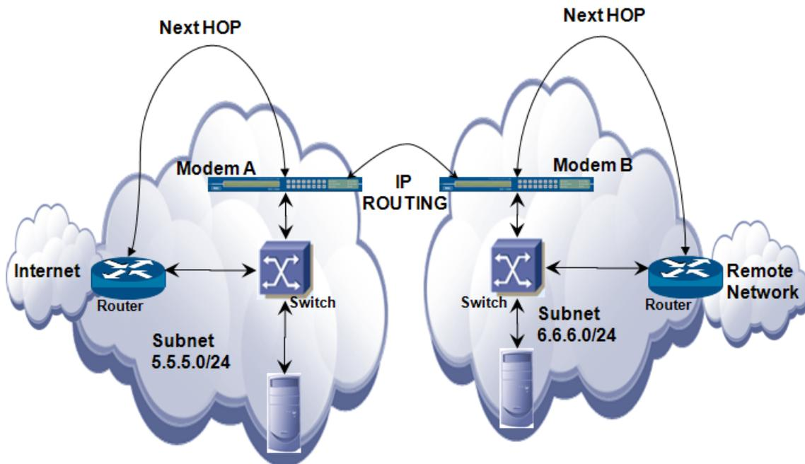
Figure 6 - IP Routing
