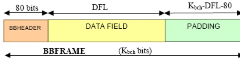
Figure 113 - Baseband Frame Structure (Source: EN-302307)
