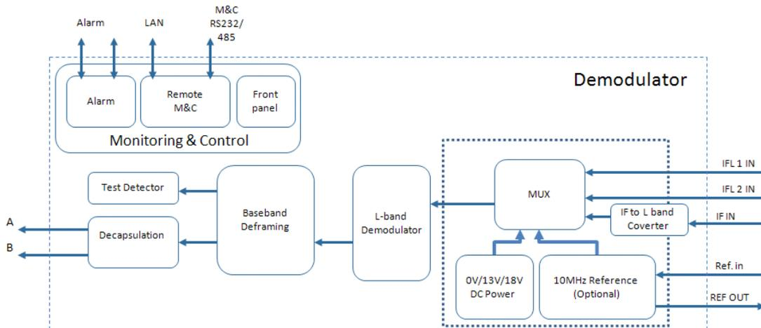
Figure 56 - Combined block diagram – L-band
