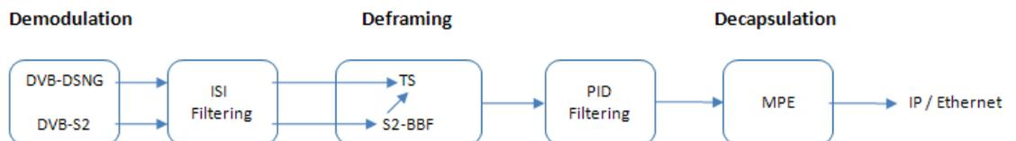
Figure 68- Demodulation, Deframing and Decapsulation
