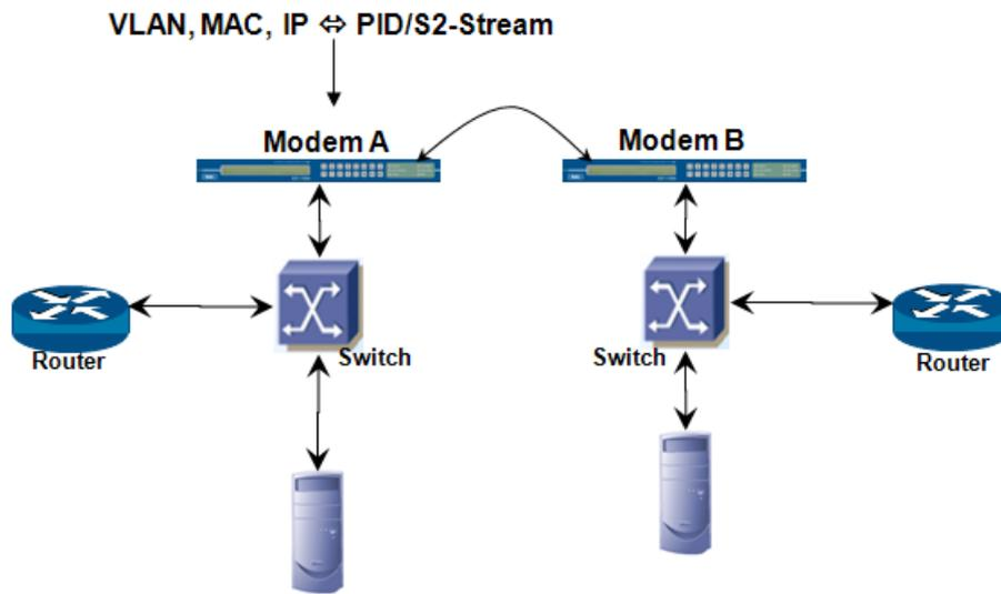
Figure 2 – Ethernet Bridging VLAN to TS PID or DVB-S2
