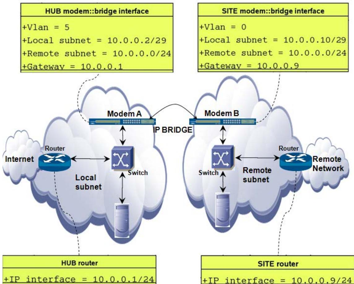
Figure 4 - IP Bridge Configuration
