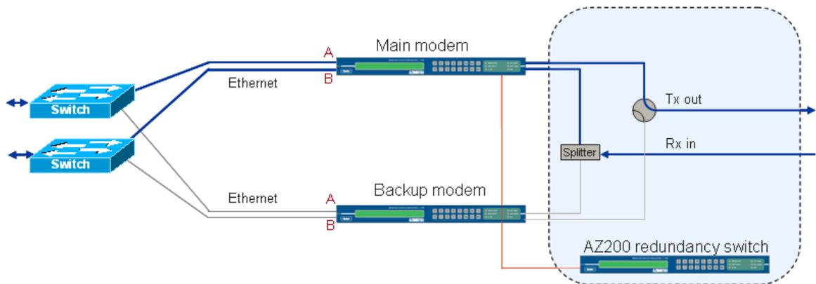
Figure 103 - example of Equipment and Port Redundancy Configuration
