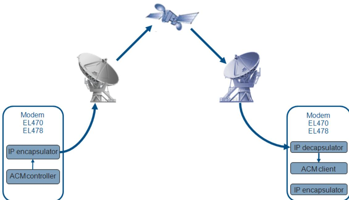
Figure 85 - In-band Forward Signalling
