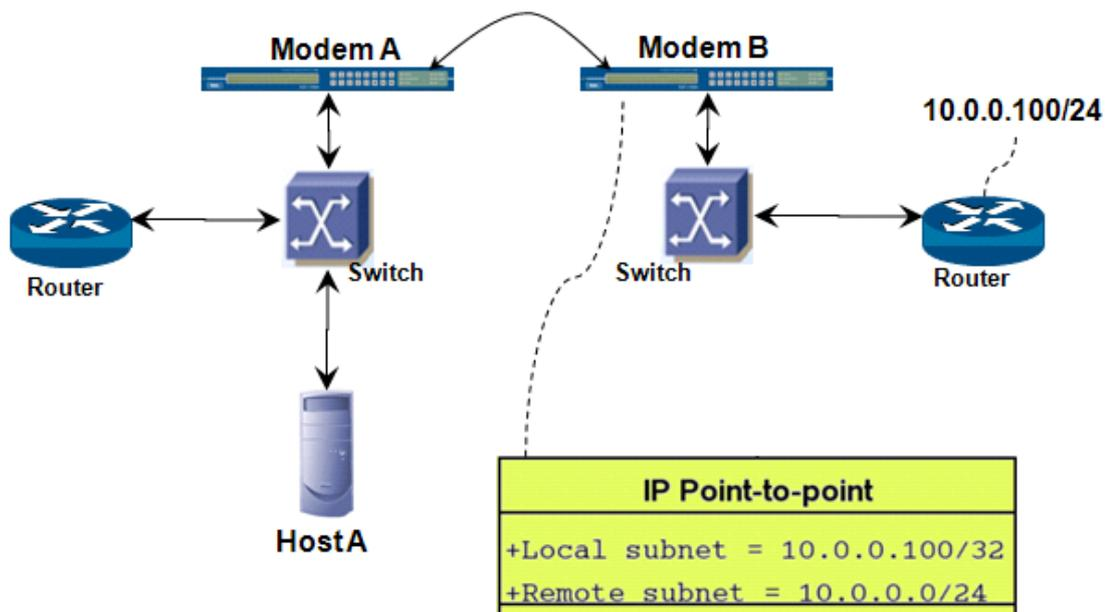
Figure 5 - Point to Point Set-up
