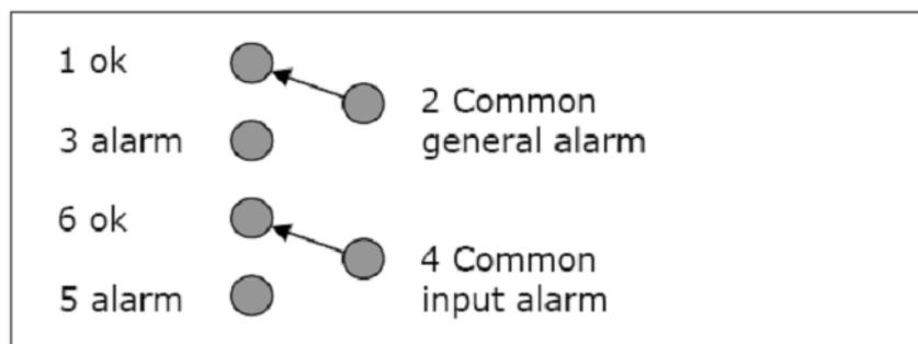
Figure 20 - Contact Closure Alarm Connections of the EL170 and EL470
