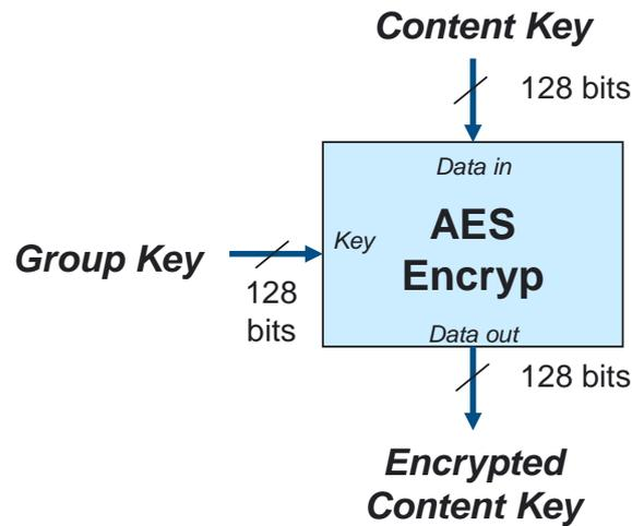
Figure 120 - Process to Encrypt a Content Key with a Specific Group Key in 128-bit Mode
