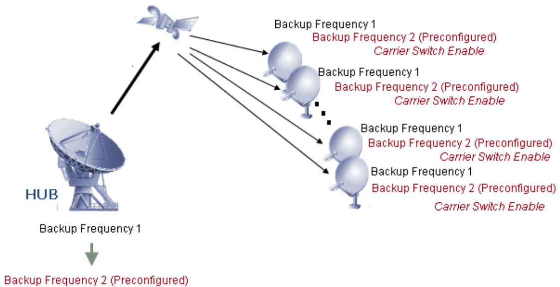
Figure 109 - Backup Carrier in the Network
