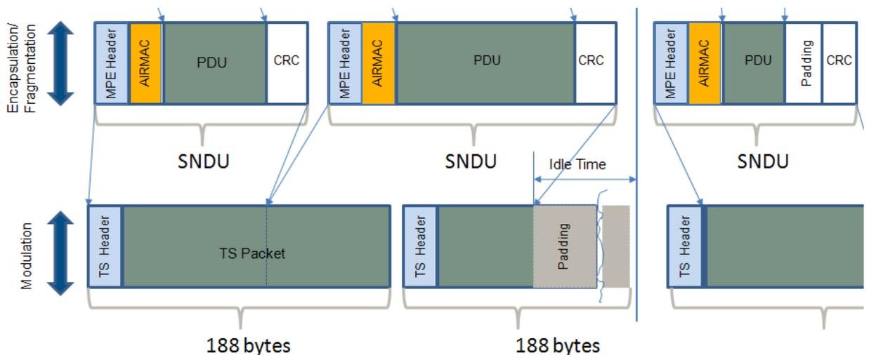
Figure 66- MPE Encapsulation of IP packets with Time Out
