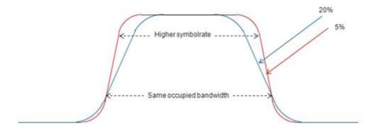
By lowering the roll-off factor and accordingly increasing the symbol rate, the throughput can be increased while maintaining the same occupied (leased) bandwidth.
