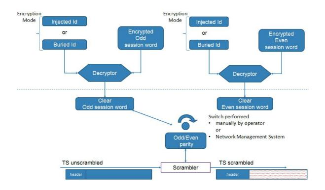
The key management structure can be split up into two parts, distribution of clear session words over a secure channel (bottom part) and distribution of Encrypted session words over a non-secure channel (top + bottom part). Both distribution methods are explained in the following sections.
