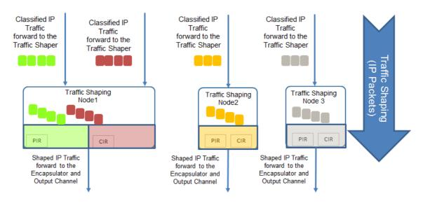
Per classified traffic node, traffic shaping can be performed.
