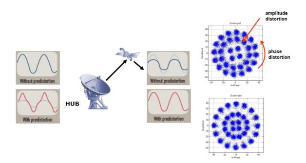
Newtec M6100, MDM6100, MDM6000 Modulators equipped with the Equalink<sup>™</sup> feature contain both linear- and non-linear pre-distortion functions, which can be individually enabled/disabled.
