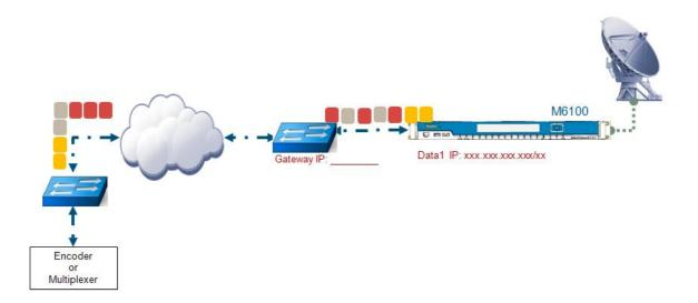
In this use case, the modulator is connected to a video encoding system that generates a TS over IP. To combat RFI we want to insert a Network ID into the TS. This TS is modulated in DVBS -2 QPSK and transmitted over satellite to set-top boxes in a DTH (Direct-To-Home) network.
