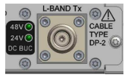
The connector used is an N-connector 50 Ohm (Female).
