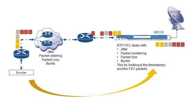
The insertion of SMPTE-2022 FEC packets is based on a two dimensional XOR (exclusive or) algorithm.
