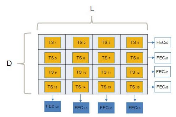
When the transport streams are aligned in the matrix the XOR function is applied to compute the FEC packets per column and row.
