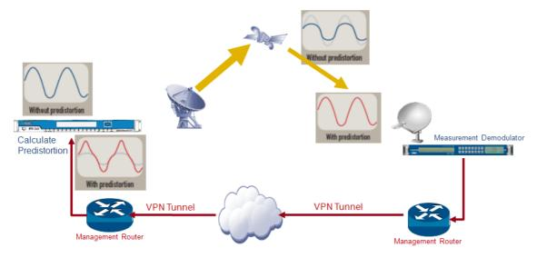
The automated Equalink<sup>™</sup> calibration is done by performing measurements between the M6100 and a Newtec demodulator or modem.
