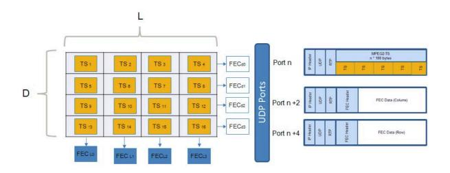
The M6100 Broadcast Satellite Modulator has all hardware on board to support L(column) and D (Row FEC) up to 20 where L\*D<=100.
