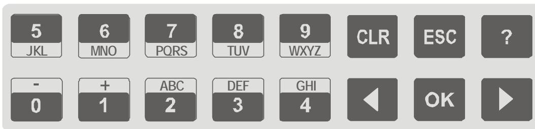
The 16-frontpanel keys allow the operator to navigate in the menus and change parameters.
