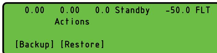
This menu controls system parameter backup to floppy disk. See **Section 8.3.1, "ACU Parameter Back-up To 3.5" Floppy Disk" on page 8-2** for instructions on this function.
