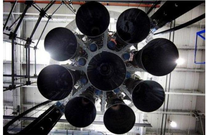
The new layout also provides individual protection for each engine, and further protects other engines in case of an engine failure. It significantly reduces both the length and weight of the Falcon 9 first stage. With this design, Falcon 9 is also prepared for reusability – the Octaweb will be able to survive the first stage’s return to Earth post-launch.
