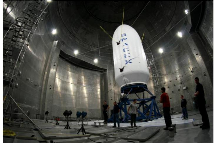
There are two halves to the fairing. One side is passive, and one is active with all actively controlled systems.
