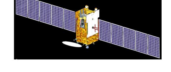
GSAT-24 is a Ku-band 4-tonne class communications satellite built for NSIL by ISRO. This satellite will provide high-quality television, telecommunications and broadcasting services and will meet the DTH needs of Indian customers. GSAT-24 is configured on ISRO's proven I-3k Bus with a mission life of 15 years.
