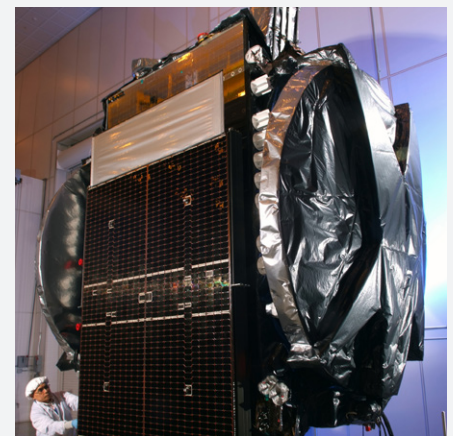
Intelsat 15 in Orbital ATK's Dulles, Virginia satellite manufacturing facility
