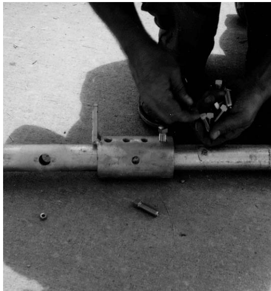
Figure 3-15: Azimuth Strut-Bracket Assembly
