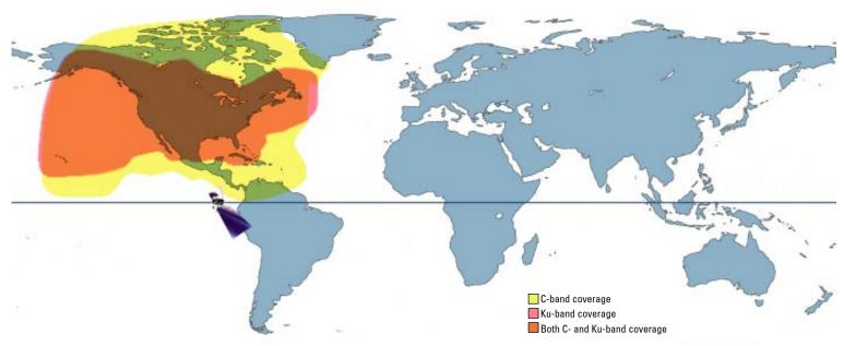
Launched in September 1997 at 87° W.L., AMERICOM-3 (AMC-3) is the third of SES AMERICOM's A2100 hybrid C- and Ku-band satellites.
