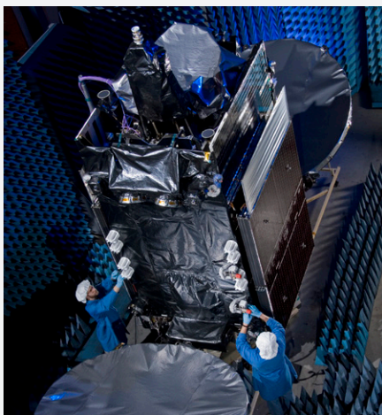
Intelsat 11 undergoes testing in the Antenna Range at Orbital ATK's satellite manufacturing facility in Dulles, Virginia.
