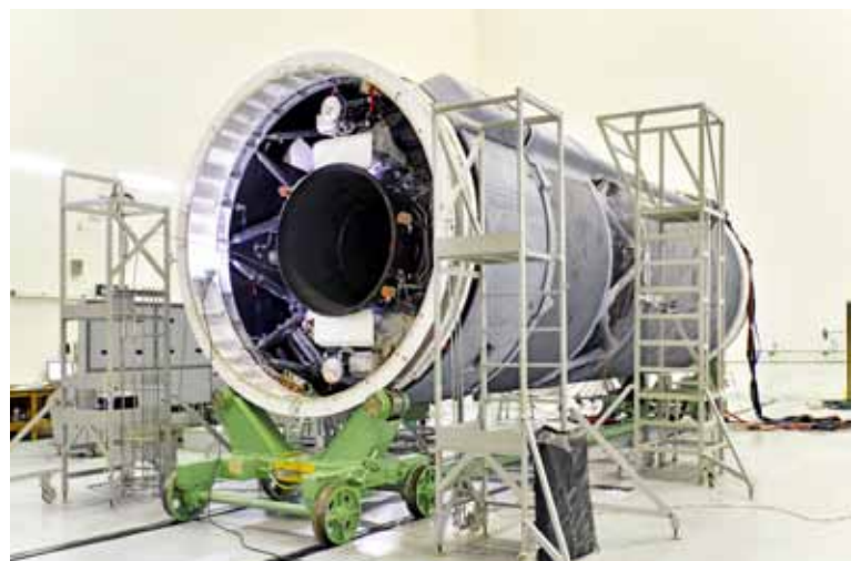
Indigenous Cryogenic Upper Stage of GSLV-F09 at Stage Preparation Facility
