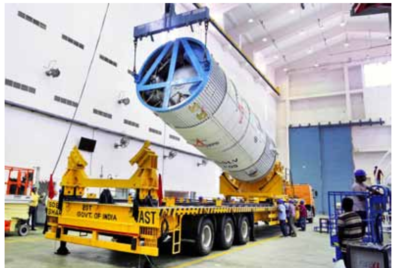
Hoisting of the GSLV-F09 second stage during vehicle integration
