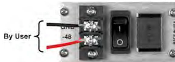
Figure 4-11. Apply DC Power to the Unit
