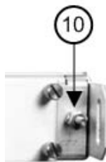
Figure 4-12. Unit Ground Connection
