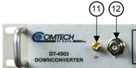
Figure 4-14. Front Panel Sample Test Point Connections
