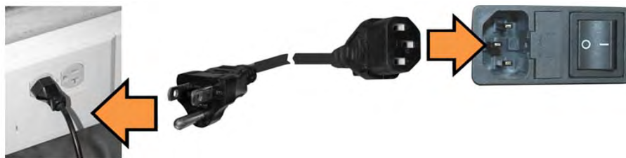
Figure 4-9. Apply AC Power to the Unit
