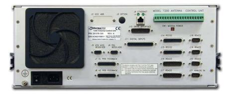
The rear panel of the 7200 accommodates all I/O for the unit including drive interface, serial communications, axis interfaces and communications with other tracking equipment.
