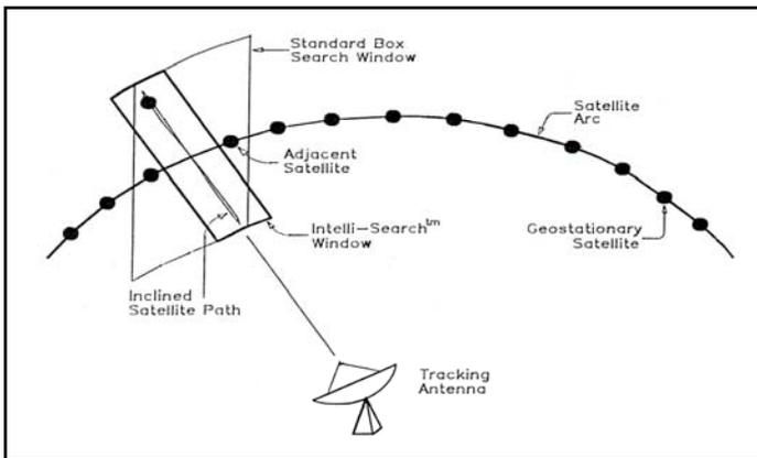
satellite has been stored in the RC2500, finding it again is as easy as locating a fixed satellite. Simply move to Auto mode, select the satellite from the list of those available, specify the proper polarization and let the RC2500 do the rest.
