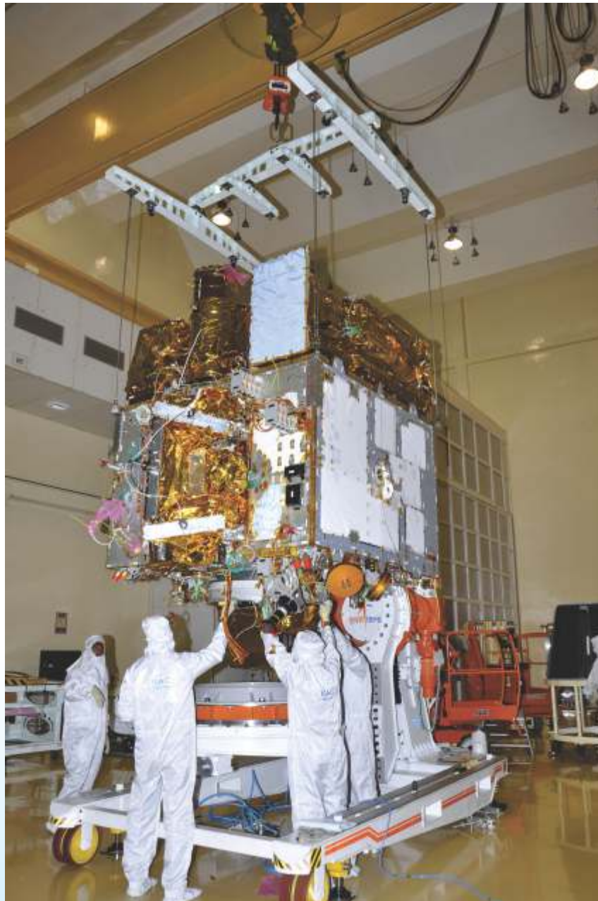
Integration of ASTROSAT in a clean room at ISRO Satellite Centre
