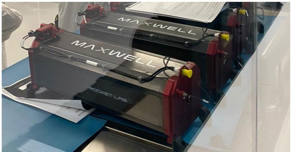
○ PLANET SUPERDOVES BEING INTEGRATED WITH ROCKET LAB MAXWELL DISPENSERS
