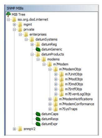
Figure F-5 – Example Tree View of the M7 Upper-Level MIB
