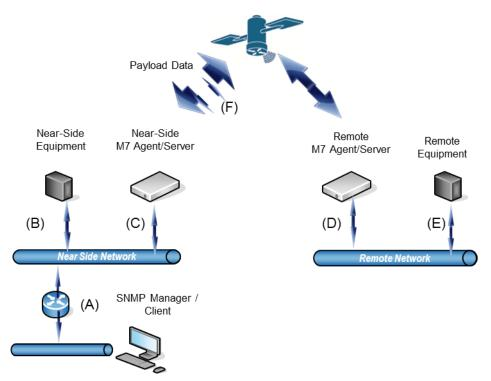
Figure F-2 - Satellite Link with SNMP
