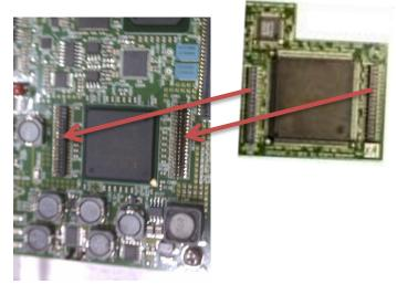
Figure 2-15 – FEC Option Card Installation
