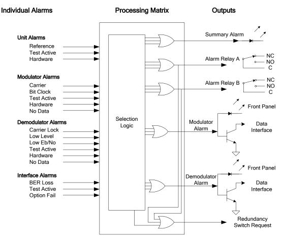
Figure 3-49 – Alarm Processing
