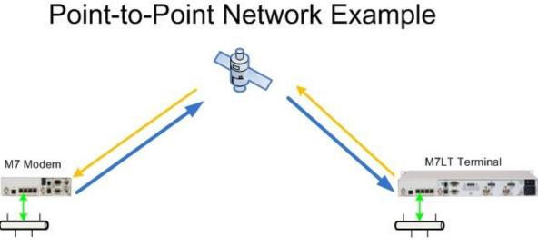
Figure 3-51 – Point-to-Point Satellite Network
