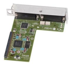
Figure 1-11 – Synchronous Serial Interface
