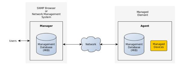
Figure F-1 – SNMP Components
