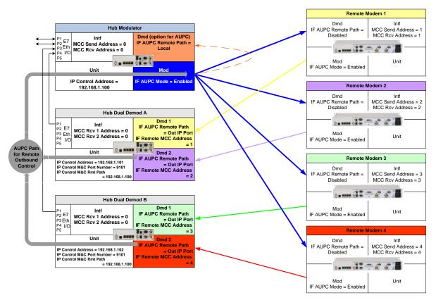
Figure 3-60 – Point-to-Multipoint AUPC configuration for a four (4) site network
