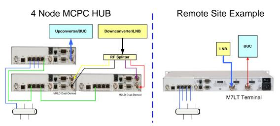
Figure 3-53 – Four site PtMP Hub and one Remote site example
