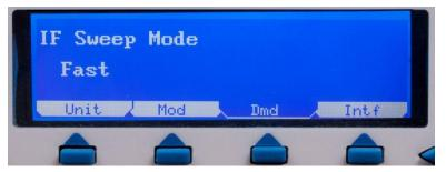
**Comd: IF Sweep Mode – Fast or Search>** "Fast" enables fast acquisition mode. Search mode is only used with very low symbol rates where multiple carriers can be within the IF Sweep Range. Should be set to "Fast" under normal conditions.
