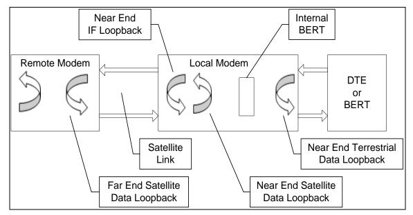
Figure 4-1 – Loopback Block Diagram
