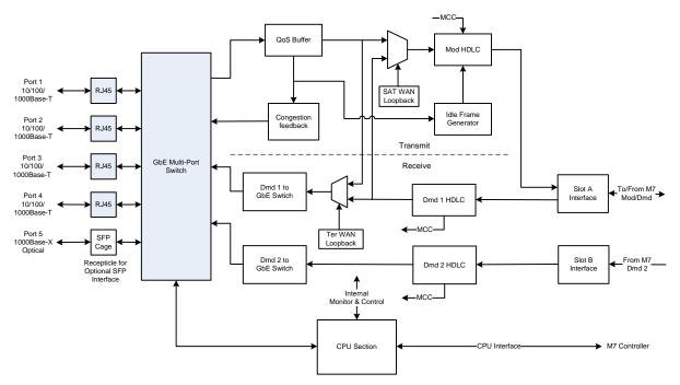
Figure 3-50 – Express Ethernet Interface Block Diagram
