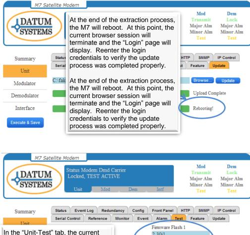
In the "Unit-Test" tab, the current updated firmware will show in either "Firmware Flash 1 or 2" and display "Running" to indicate it is the operating firmware. The previous firmware will be maintained in the other flash location and can be called up if there is an issue with the new update.
