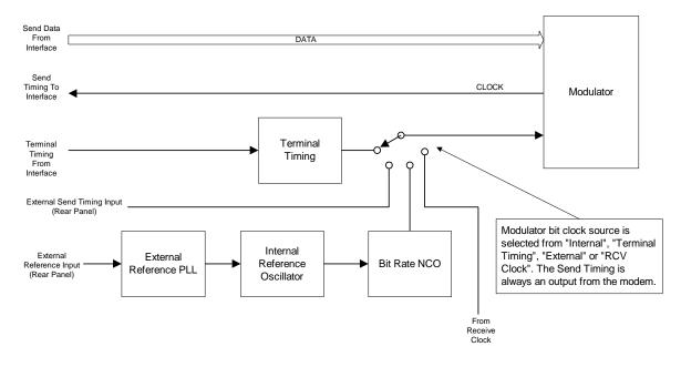
Figure 3-56 – Modulator Clock Source Options
