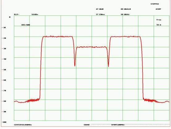
Figure 1-10 – Carrier Alpha = 0.08, 1Msps x1.10 Carrier Spacing
