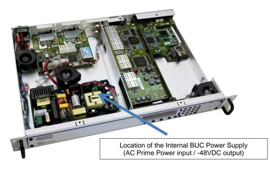
Figure 2-6 – M7LT Internal BUC Power Supply (AC version shown)
