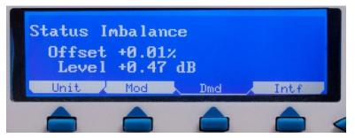
**Status: Imbalance – Offset>** Shows the frequency offset imbalance between the far end carrier and the echo carrier as a percentage of the receive symbol rate. For best performance the two carriers should be close together in frequency, typically the difference should be less than 1% of the symbol rate.
