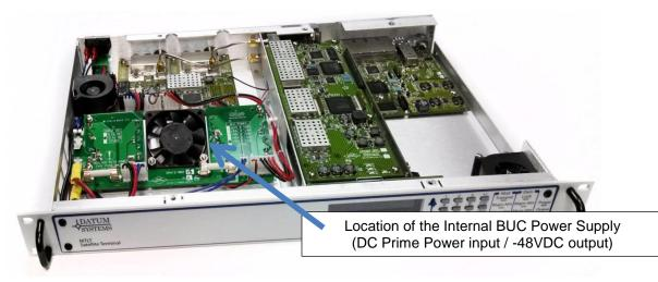
Figure 2-7 – M7LT Internal BUC Power Supply (DC Version)
