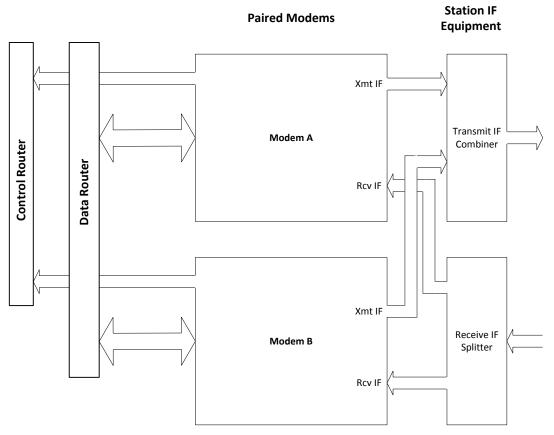
Figure 3-61 – M7 Connections for 1:1 Redundancy
