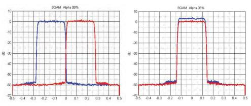
Figure 1-20 – Smart Carrier Bandwidth Savings of 50%
