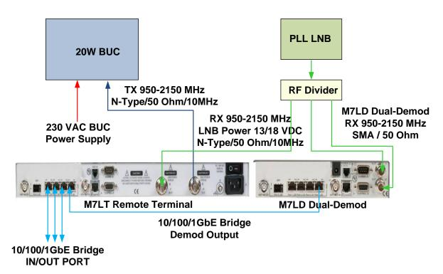
Figure 3-55 – Configuration of a Mesh network site with a spare demodulator
