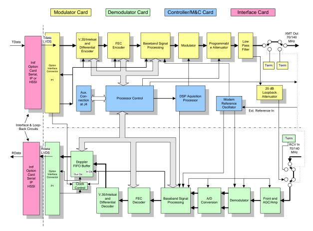
Figure 1-8 – Modem Block Diagram
