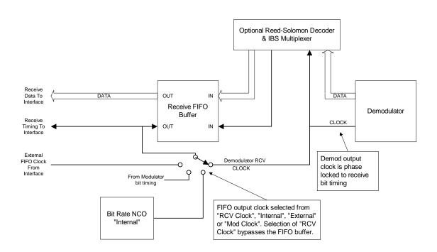
Figure 3-57 – Demodulator Clock Source Options
