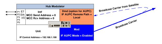
Figure 3-59 – Hub Modulator with optional AUPC Demodulator
