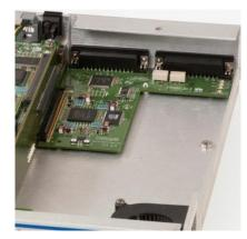
Figure 2-14 – Typical single interface card layout (Synchronous Serial Interface shown)
