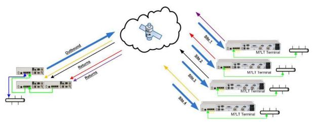
Figure 1-3 – Four (4) Site Point-to-Multipoint Network
