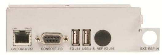
Figure 2-8 – I7 - IP Interface Rear Panel
