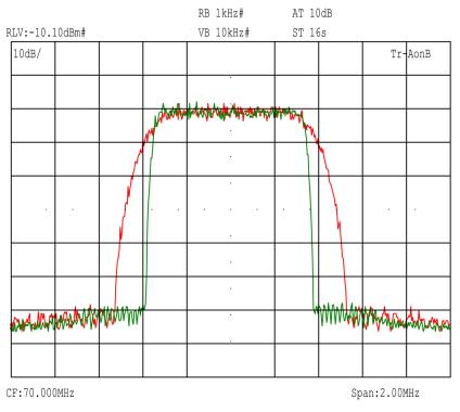
Figure 1-9 – Spectrum Analyzer Plot of 0.35 verses 0.08 Roll-off factors
