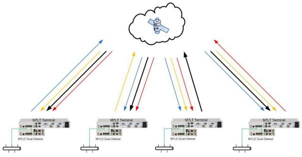
Figure 1-4 – Four (4) Site Mesh Network
