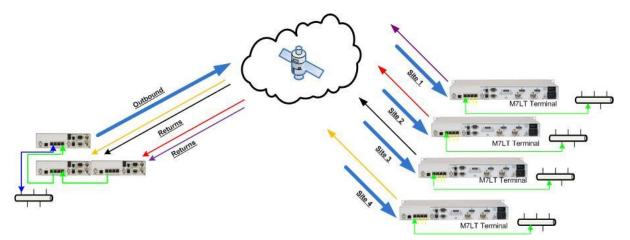
Figure 3-52 – Point-to-Multipoint Satellite Network
