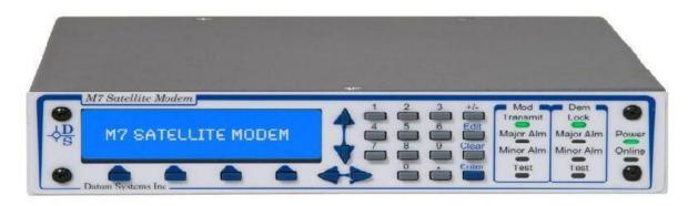
Figure 3-1 – M7 Front Panel Controls and Indicators
