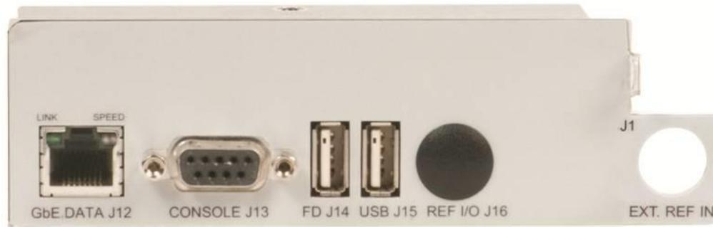
Figure 2-8 – I7 - IP Interface Rear Panel
