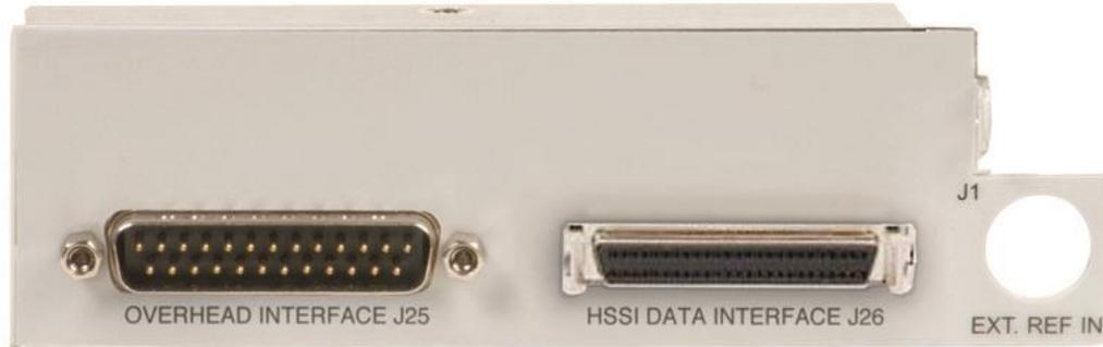
Figure 2-13 – HSSI Interface Rear Panel
