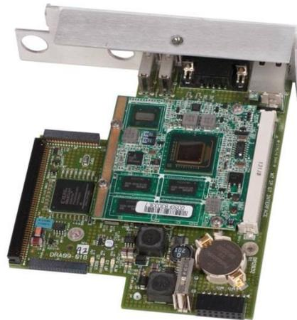
Figure 1-12 – Ethernet Interface (I7 and I7+)
