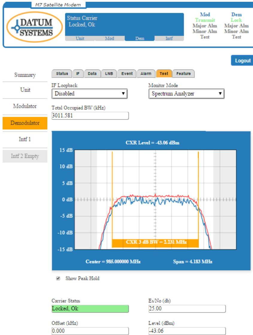
Figure 3-28 – Demodulator Monitor Spectrum Analyzer Page
