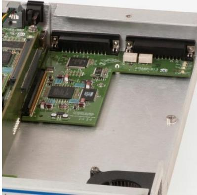
Figure 2-14 – Typical single interface card layout (Synchronous Serial Interface shown)
