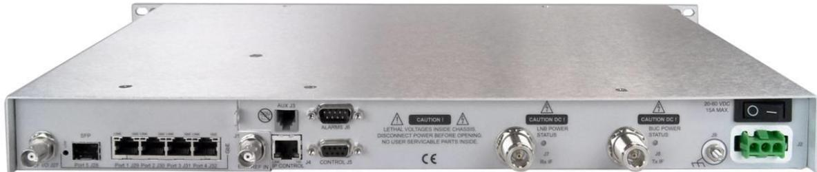
Figure 2-3 – M7LT Rear Panel with DC Prime Power Input
