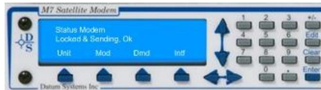
Figure 3-2 – Front Panel Matrix Navigation
