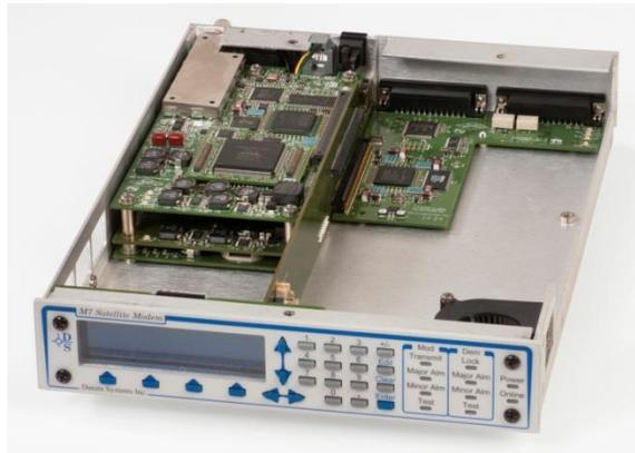
Figure 1-7 – M7 Modem Assemblies (shown with standard serial interface)
