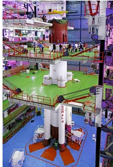
PSLV-C45 core (first) stage with four strap-ons inside Vehicle Assembly Building
