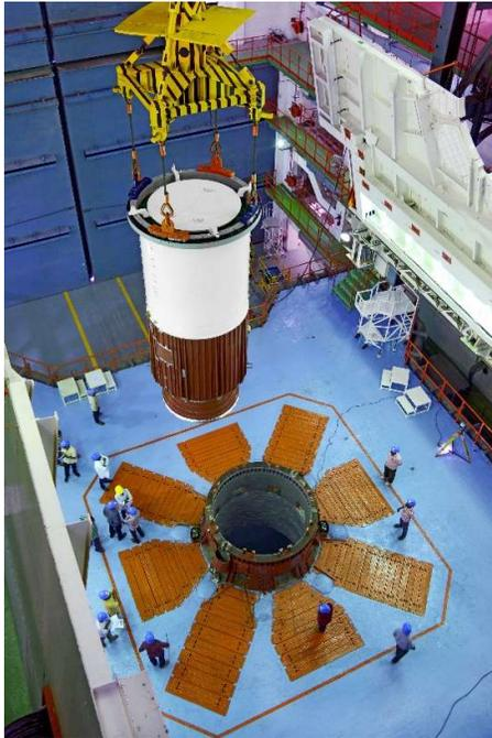
Nozzle end segment of PSLV-C45 Core (First) Stage being lowered on Mobile Launch
