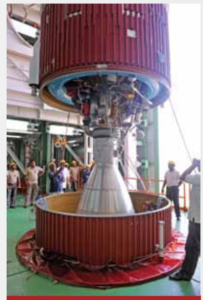
PSLV-C22 Second Stage liquid engine being lowered into the interstage
