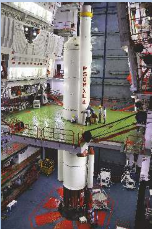
Integration of an 'XL' strap-on motor with the core stage of PSLV-C31 in progress
