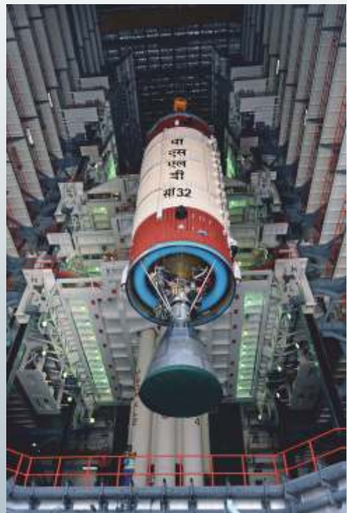
Hoisting of PSLV-C32 Second stage during vehicle integration
