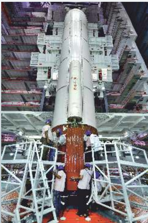
Assembly of PSLV-C32 First stage in progress
