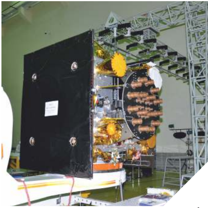
IRNSS-1F in Clean Room during its integration
