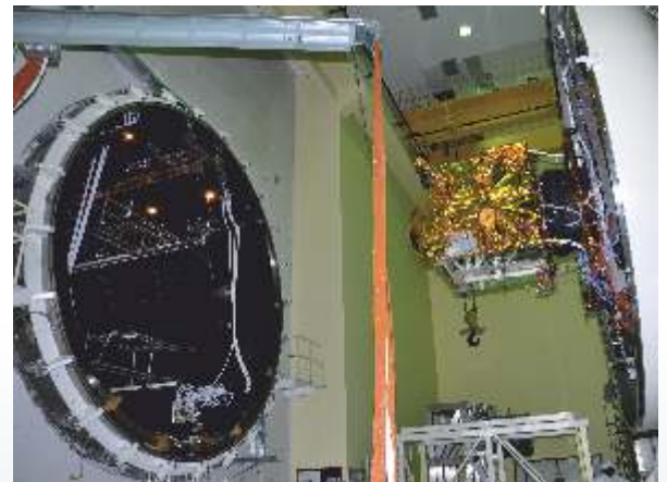
IRNSS-1F being loaded into thermo-vacuum chamber
