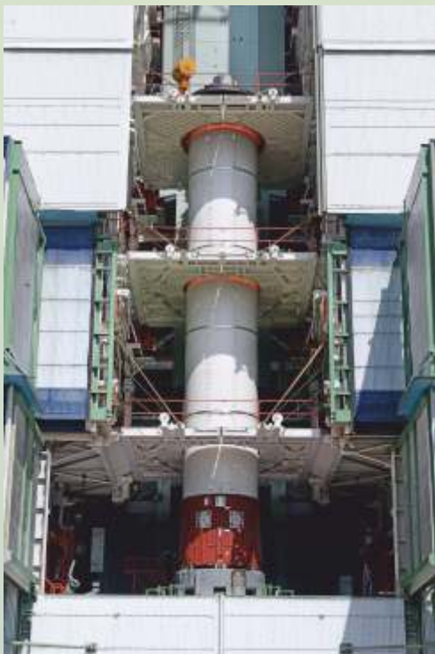
PSLV-C33 core stage integrated above the launch pedestal
