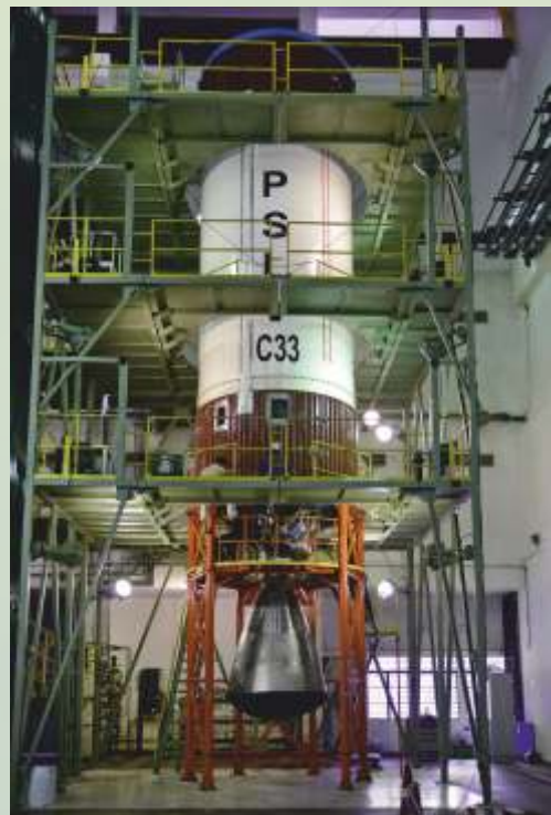
Second stage of PSLV-C33 being prepared for vehicle integration
