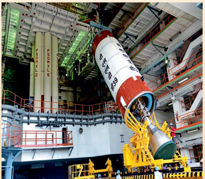
PSLV-C39 liquid second stage at the Vehicle Assembly Building during vehicle integration
