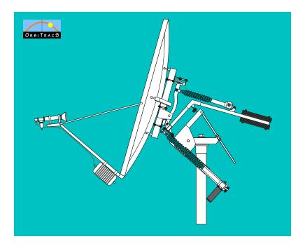
Inclined orbit tracking is performed with a second actuator in the perpendicular declination plane. The inclined tracking function is performed without any need for feed-back signals (beacon receiver, agc etc.). This thanks to a unique Orbitracs proprietary algorithm that allows open-loop tracking for many years without the need for updates, feedback or any other intervention.
