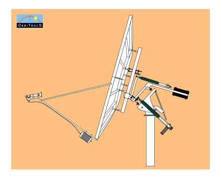
Inclined orbit tracking is performed with a second actuator in the perpendicular declination plane. The inclined tracking function is performed without any need for feed-back signals (beacon receiver, agc etc.). This thanks to a unique Orbitracs proprietary algorithm that allows open-loop tracking for many years without the need for updates, feedback or any other intervention.
