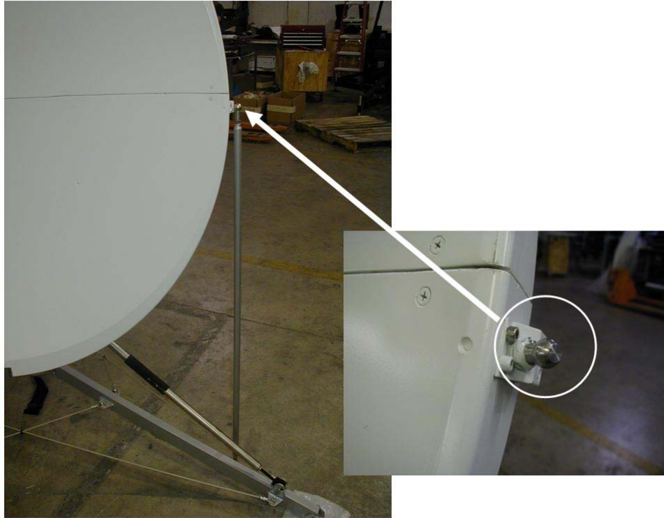
Figure 8. Feed Boom Strut Installation
