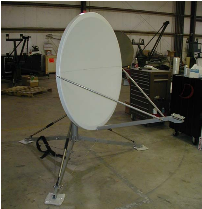
Figure 11. Feed Boom Installed
