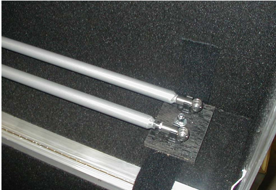
Figure 19. Feed Boom Struts in Shipping Clips
