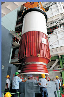
Nozzle End Segment of PSLV-C21 first stage being placed on launch pedestal
