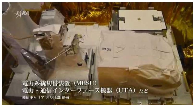
Figure 4.2-3 UTA and MBSU loaded on the EP (HTV4)
