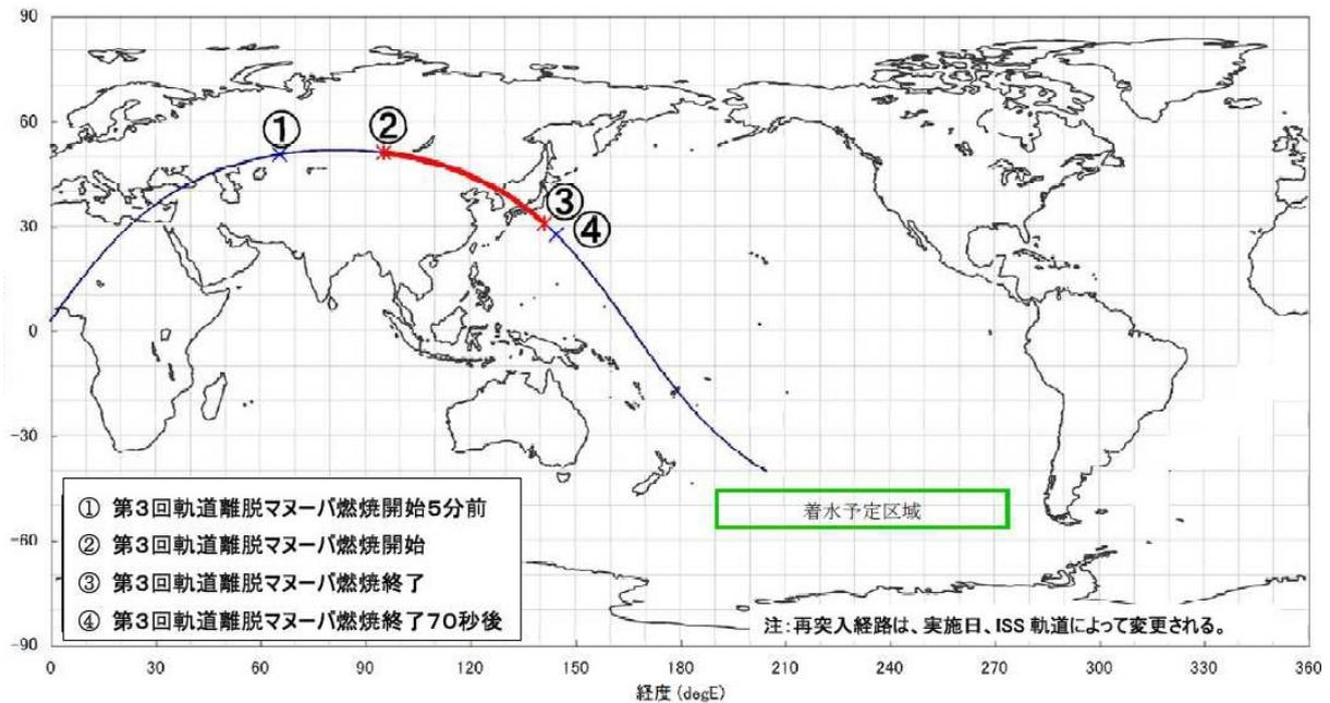
Figure A2-4 HTV's projected reentry path
