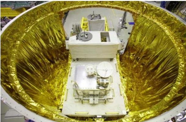
Figure A1.2-3 EP Installed into the ULC (HTV3)
