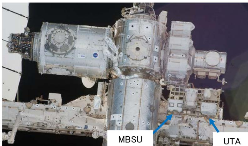
Figure 4.2.1-5 MBSU and UTA spare parts (covered in thermal insulating covers) stored on the ISS ESP-2
