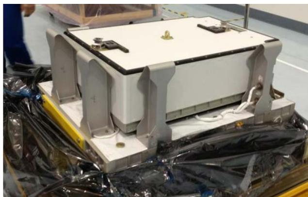
Figure 4.2.1-2 MBSU to be delivered by the HTV4
