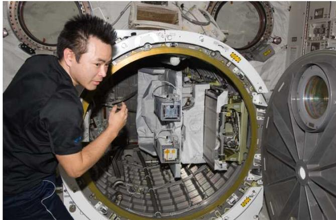
Figure A3-5 MPEP and J-SSOD installed in the Kibo's airlock
