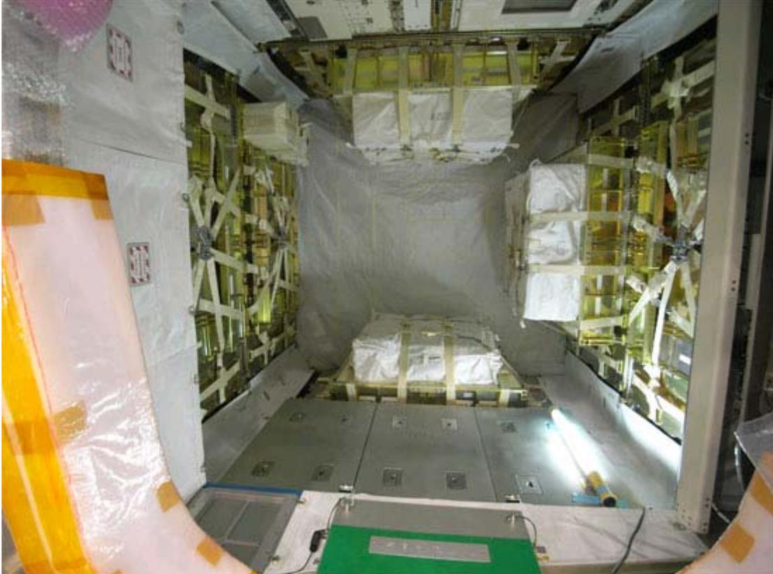
Figure A1.1-3 Rack Layout inside the HTV2 (photo taken from the hatch side, during loading)
