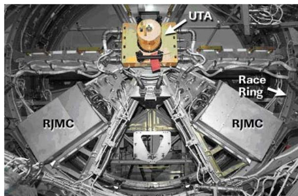
Figure 4.2.1-4 UTA installed to the center of SARJ
