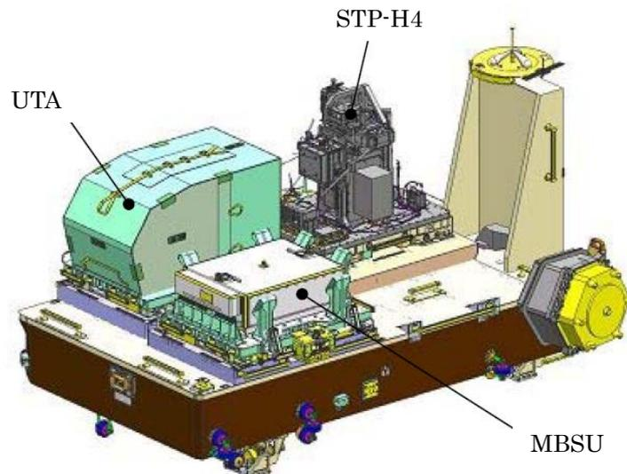
Figure 1.3-3 Cargo layout on the Exposed Pallet (NASA/JAXA)
