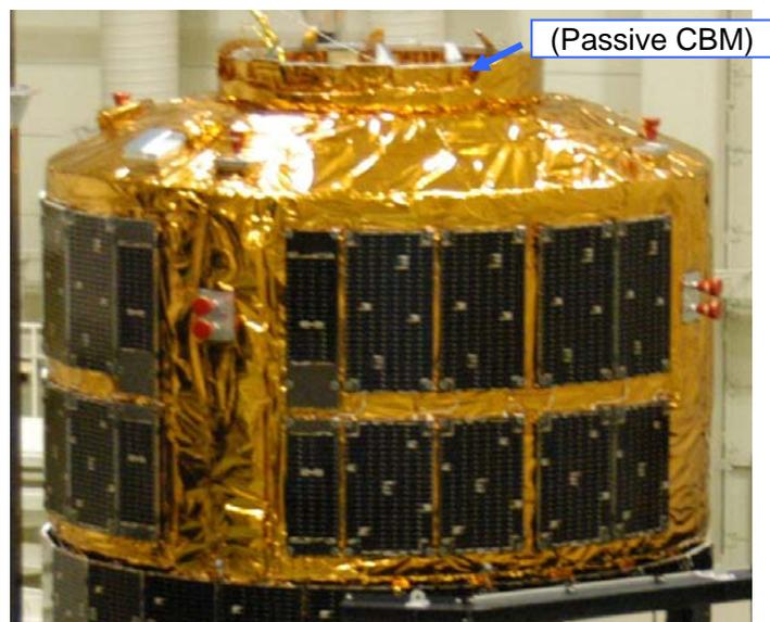
Figure A1.1-1 PLC exterior (HTV1)
