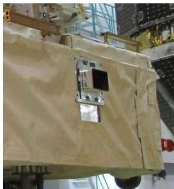
Figure A1.3-6 HTV Berthing Camera System (HBCS)
