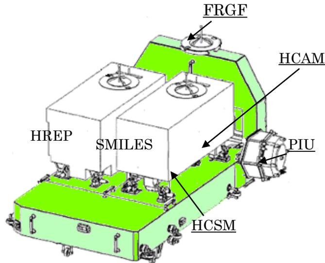
Figure A1.3-2 Exposed Pallet for EF Payload (Type I)
