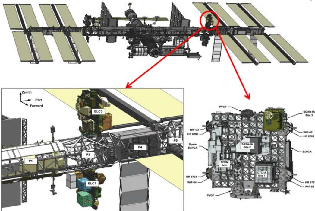
Examples of installation location of unpressurized cargo (ELC-3)
