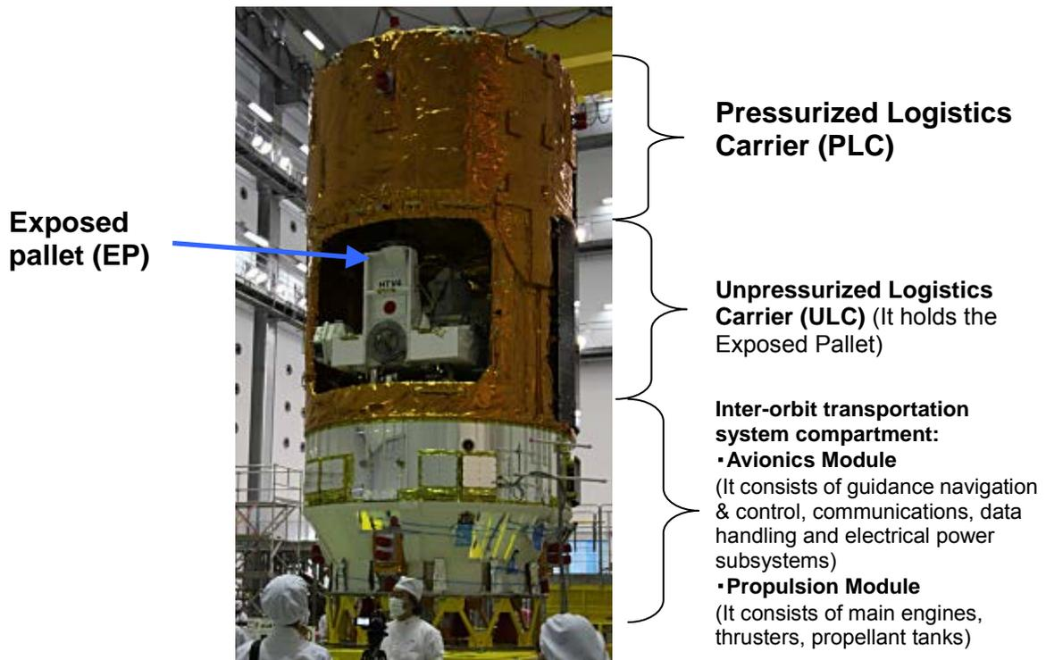
Figure 1.1-1 Configuration of “KOUNOTORI” (photo: HTV4)
