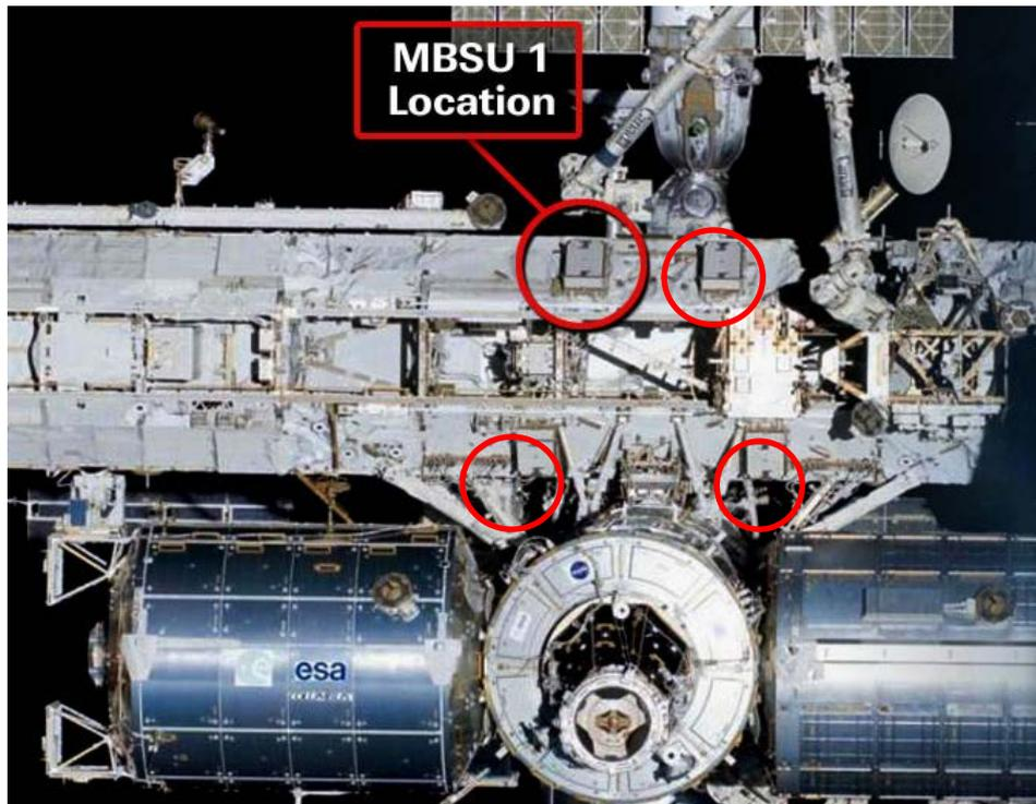
Figure 4.2.1-1 Four MBSU installed on the S0 truss of the ISS
