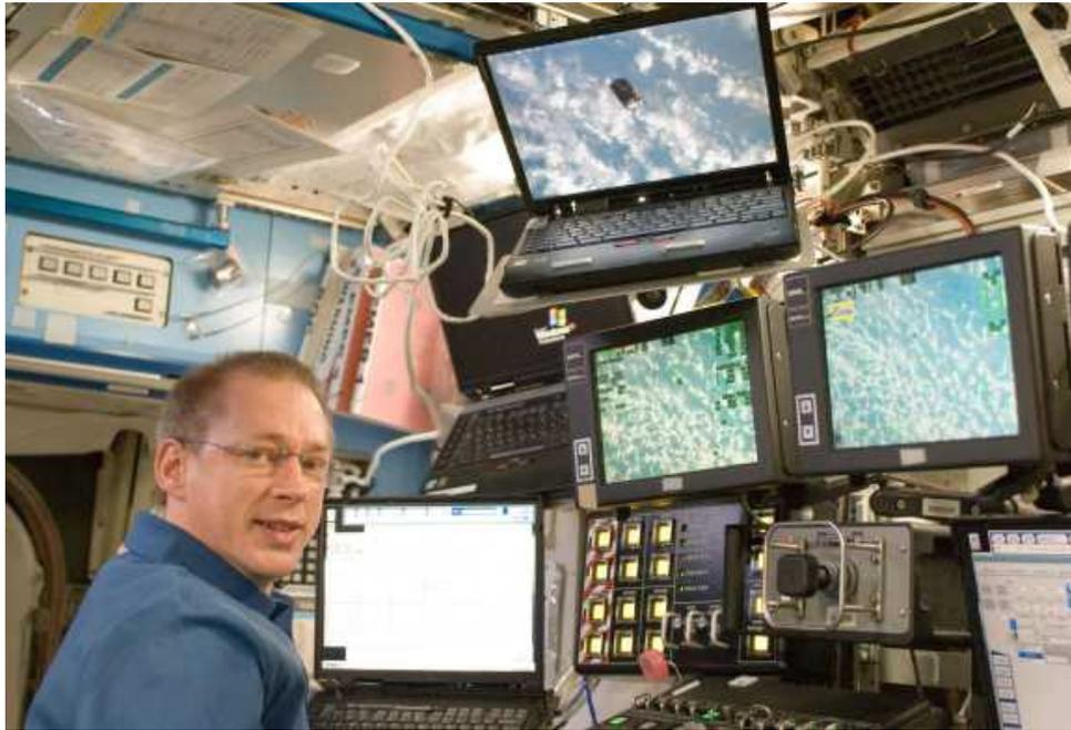
SSRMS Console used to grapple the HTV (HTV1 mission) (Credit: JAXA/NASA)
