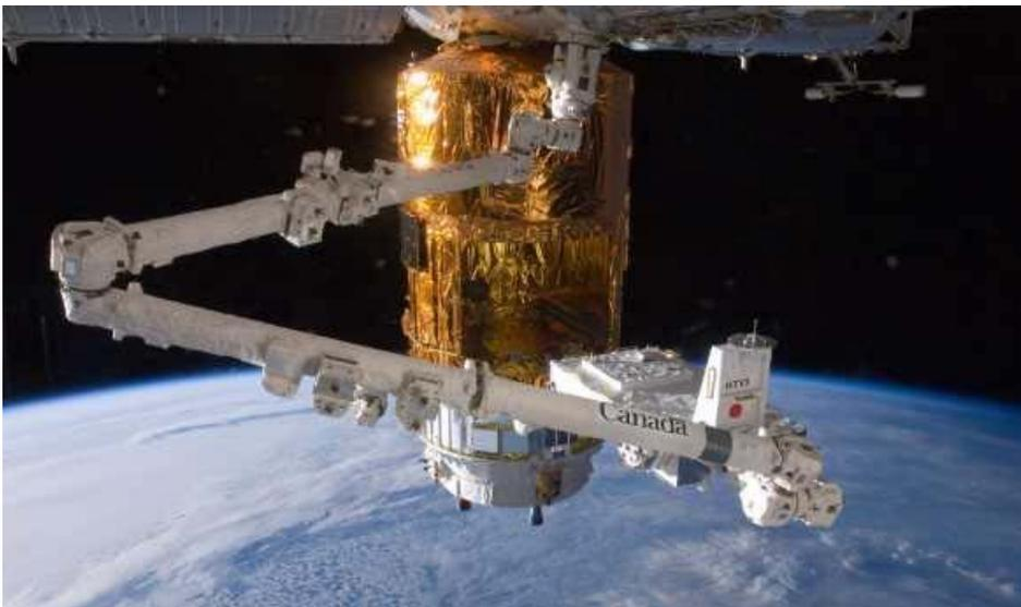
EP being reinstalled into the ULC (HTV3)
