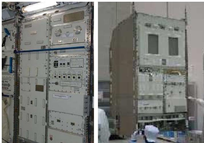
Figure A2-11 Gradient Heating Furnace (GHF), Multi-purpose Small Payload Rack: MSPR (Delivered by the HTV2)
