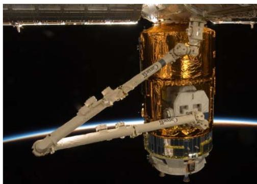
The SSRMS removing the EP from the ULC
