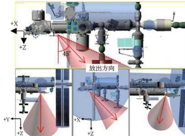
Figure A3-7 Images of CubeSats release operations and release angles
