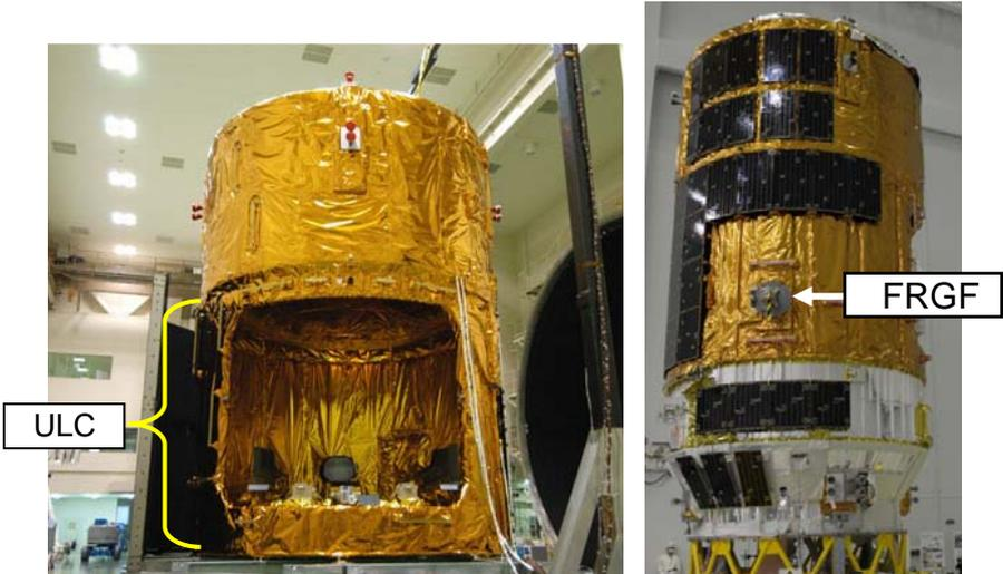
Figure A1.2-1 ULC before Installation of the EP (HTV1)
