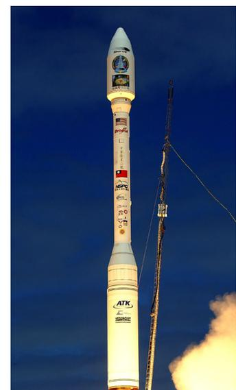
The Minotaur-C launch vehicle is a ground-launched variant of Orbital ATK's highly successful Pegasus air-launched space booster.
