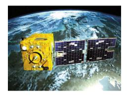
**ESTCube-1:** Technology demonstration satellite launched for the National University of Tartu in Estonia. Its main mission is to measure and test the loads that could be applied to electric solar sails, a new concept for propulsion.
