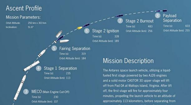
The Antares space launch vehicle, utilizing a liquidfueled first stage powered by two AJ26 engines
