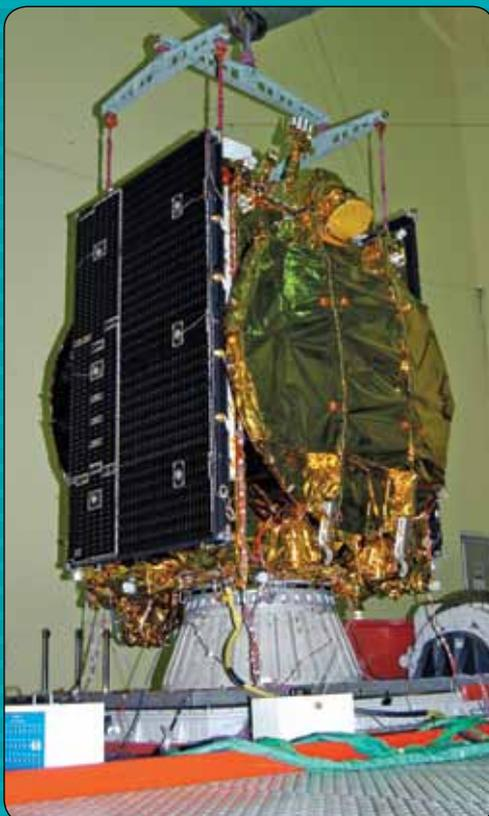
GSAT-14 undergoing vibration test
