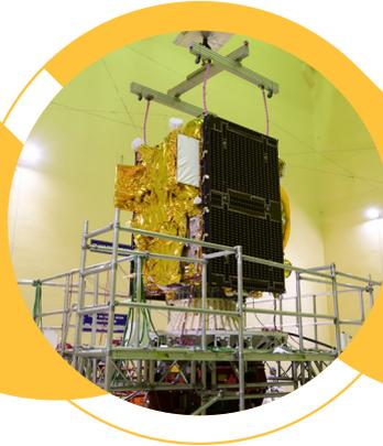
**NVS-02 undergoing Solar Panel Deployment Test**
