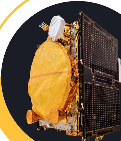
Like its predecessor, NVS-02, the second satellite in the NVS series is configured with Navigation payload in L1, L5 and S band in addition to ranging payload in C-band. It is configured on standard I-2K bus platform with a lift-off mass of 2250 kg and power handling capability of ~3 kW. It will be placed at 111.75°E replacing IRNSS-1E. NVS-02 uses a combination of indigenous and procured atomic clocks for precise time estimation.
