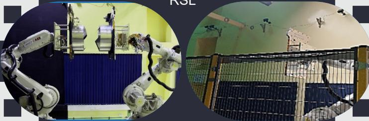
Rendezvous Simulation Lab (RSL) for validating onboard algorithms with real-time simulations. Detailed characterisation tests at sensors level have been carried out in addition to system level tests.
