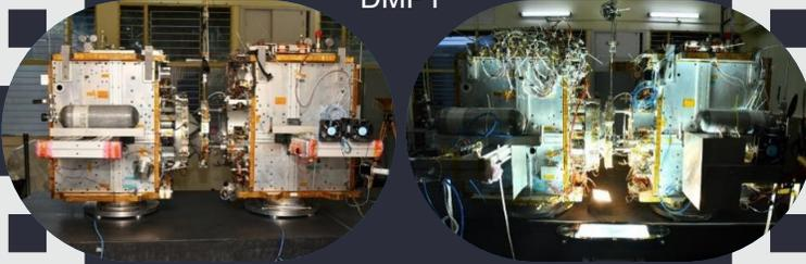
Docking Mechanism Performance Test (DMPT) for testing final phase of Autonomous Rendezvous Docking and Undocking Sequence (ARDUS)
