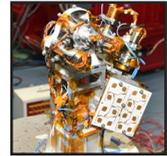
**Flexible Solar panel** consists of Foldable solar panel substrate, GFRP tube, CFRP honeycomb rigid end-panel.
