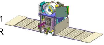
The satellite carries a host of new technology developments in satellite mainframe systems like an Integrated Avionics system - Communication, Baseband, Storage and Positioning (CBSP) Package, Structural panel embedded with PCB, embedded battery, Micro-DGA (Dual Gimbal Antenna), M-PAA (Phased array antenna) and Flexible solar panel & Nano star sensor etc for onboard Technology Demonstration. The satellite is slated for launch by Small Satellite Launch Vehicle (SSLV)-D3.
