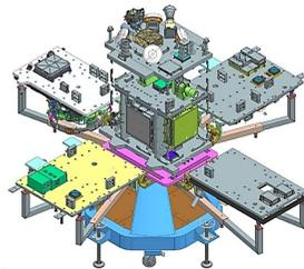
**Micro-Dual Gimbal Antenna (mDGA)** having rotational speed of 6°/s and pointing accuracy of  $\pm 1^\circ$ .
