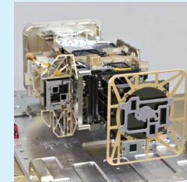
EXIS monitors solar irradiance in the upper atmosphere and detects solar flares that could interrupt communications and reduce navigational accuracy, affecting satellites, high-altitude airlines, and power grids on Earth. On board EXIS are two main sensors, the Extreme Ultraviolet Sensor
